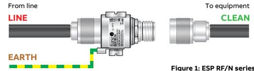
Figure 1: ESP RF/N series connection
