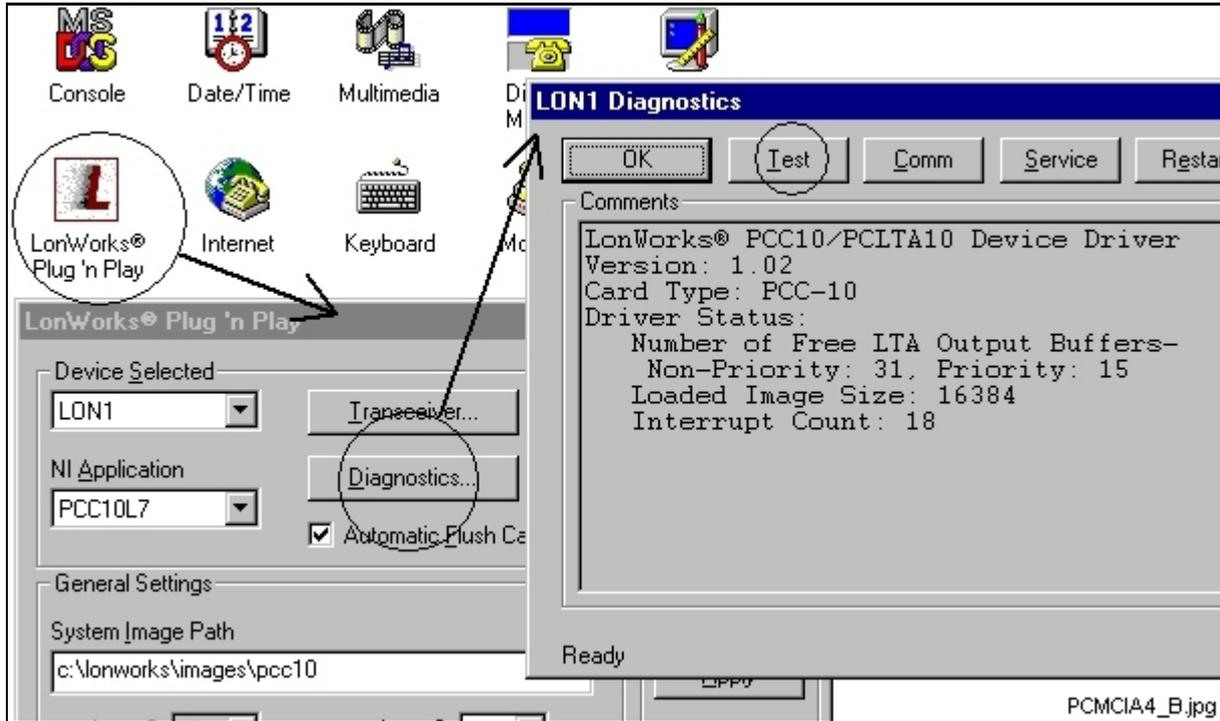
Fig. 5.2.-5 The Diagnostics dialogue can be used for testing the PCC-10 card
