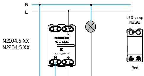
**Push-button for buzzer / bell with locator lamp**
