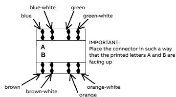
2b Wiring according to T568B:
