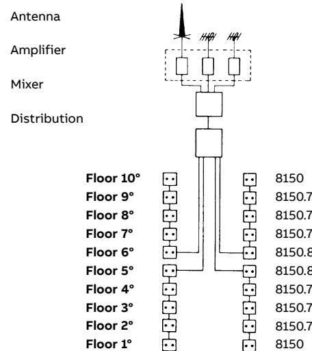
**Example:** 10 floors. The floors are divided in 2 groups of 5 floors each. The outlets are distributed according to the criteria shown in the MATV connection diagram for serial distribution up to 9 floors. The diagram above can be used in buildings up to 18 floors. For buildings with more than 18 floors and up to 27 floors, 3 groups have to be created and so on.
