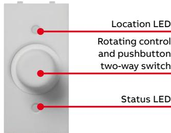
Electronic dimmer with rotary control and two-way switch for resistive loads 100-500W 230V~ -50/60Hz (visible in the dark).
