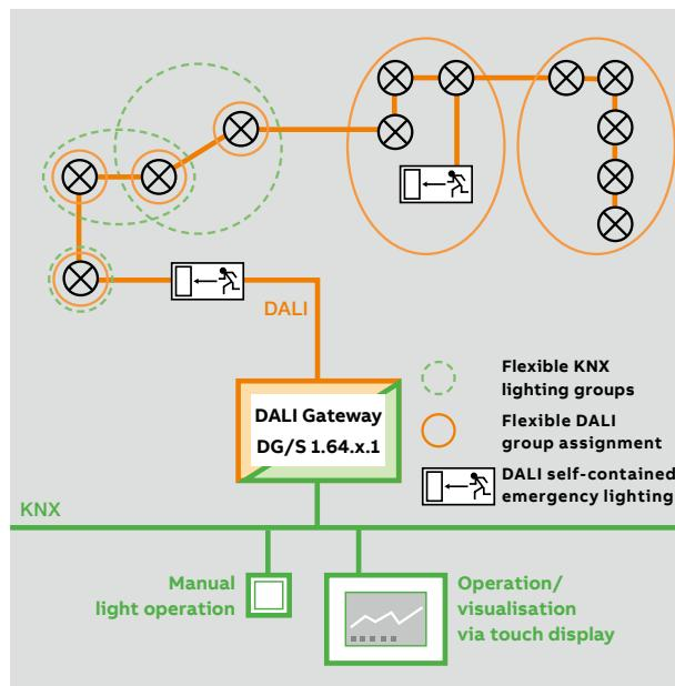
Both basic Gateways are equipped with emergency lighting function, support the DALI standard EN 62386-202 that specifies DALI emergency lighting (self-contained).
