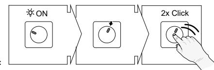
To adjust an established luminosity connection the following points must be executed:
