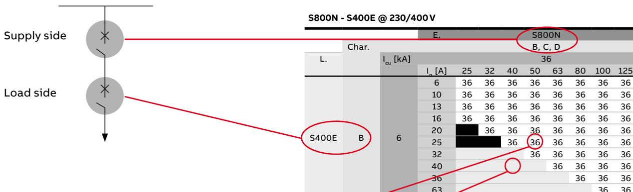
Example 1: With a S800 nominal current 50A is a Back-up protection till a nominal current of 25A to a S400 given. The Back-up protection ist till 36kA.
