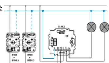
8130.2 with auxiliary buttons (8144.2, 8104.5) and two lamps.
