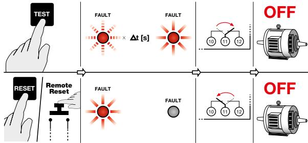
On RD3P version, a no trip test can also be performed by simultaneously pressing the front test and reset buttons for 3 seconds. In this case, the output contacts will not switch, as shown in the figure below:
