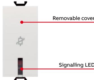
This device provides protection for power supply sockets for all types of household appliances and in particular for those containing electronic components (Hi-Fi, TV, computers, video recorders, programming mechanisms, cash registers etc.) from damage caused by over-voltages present in power supply networks.
