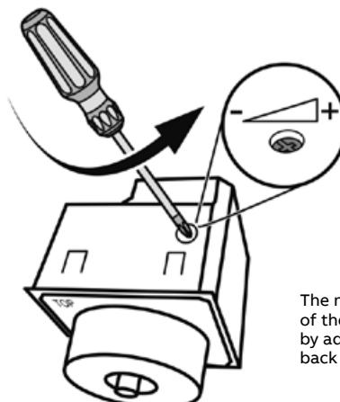
The minimum brightness of the dimmer can be set by adjusting the on the back side of the device.
