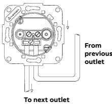
**Important:** the connection of the TV outlets in serial distribution must be carried out according to the figure on the left. The cable coming from the previous outlet is connected in the right terminal and the cable going to the next outlet in the left terminal.
