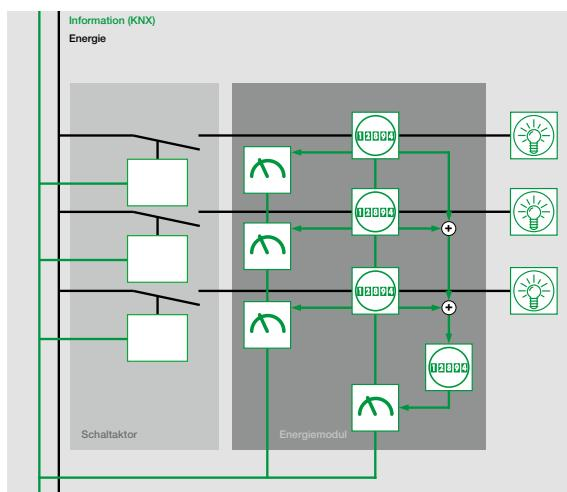
The Energy Module can record the energy consumption for the individual devices. It is used particularly when upgrading existing KNX systems and wherever energy measurement is required without switch functions. It facilitates a detailed and transparent insight into the energy consumption of a building. The current meter values can be sent and evaluated.
