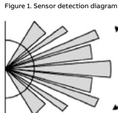
Cross section diagram showing the detection area
