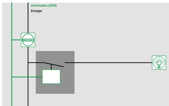
Electronic energy meters make the current energy values available on the KNX bus system in conjunction with a KNX interface. The measured data can be intermediately stored, evaluated and visualized from here.
