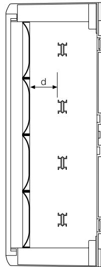
The distances of the DIN rail from the Panel depend on depth adjustment made through rail mountings.
