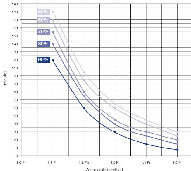
If a transformer is used with an intermittent duty cycle, it can be sized according to the formula:
