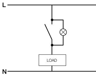
Warning light on when the switch is OFF (if the switch is in the ON state, the warning light is off while the load is ON).
