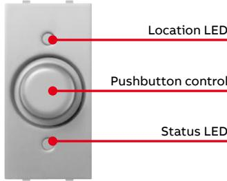
Electronic dimmer with pushbutton control for resistive and inductive loads 60-500W 60-500VA 230V~ -50/60Hz (visible in the dark).
