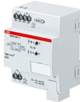
The DALI Gateway (2-fold) Basic and Premium can install up to 2 x 64 DALI devices both via 2 x 16 flexible DALI (orange lined group) and KNX lighting groups (green dotted lined group), each with one or more DALI participants. Control and Monitoring via KNX. Control and status feedback can also be carried out via Broadcast. 2 x 16 independent Lighting scenes are available.
