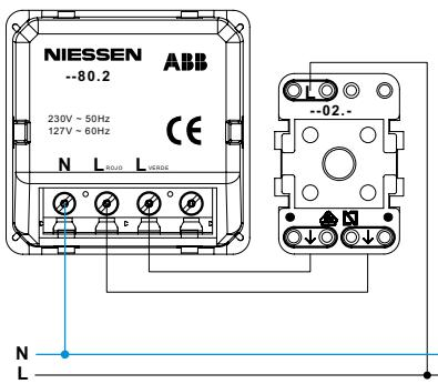
where it is located. Installed in conjunction with a conventional switch, it makes it possible to have an indicator to indicate free or restricted passage, as relevant at any time (Figure 1).
