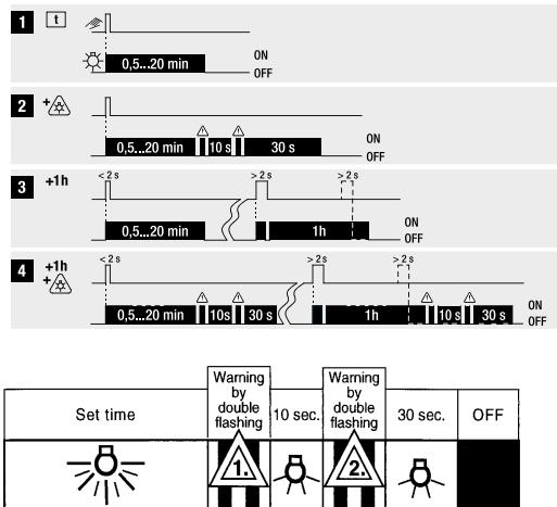
Function: Latching relay, Latching relay with returning time
