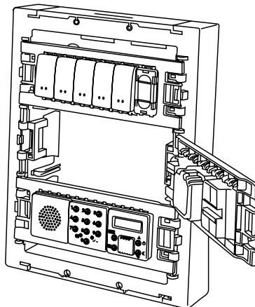
5. The mounting plate is closed by clipping.
