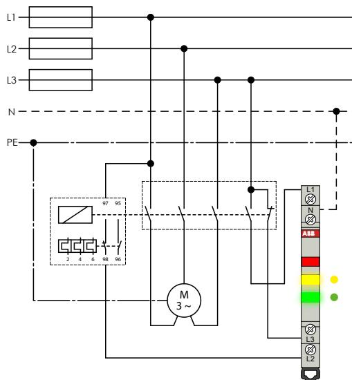
**Signaling motor interference
