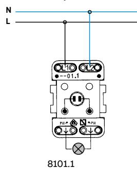
Two-pole switch with control pilot
