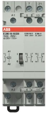
Latching Relay E290 with attached contact module E292-16-11 (additional main contact tracks) plus an auxiliary contact to externally display the switching state of the main contacts (ON/OFF).
