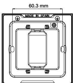
Distance between fixing screws for 1 gang frames
