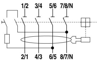
In case of installation in a 3 phase circuit without neutral, if the concatenate voltage is between 110V (170V for the 30mA version according to EN standard) and 254 V (277 V according to UL 1053) for the correct working of the test button there are two possible solutions:
