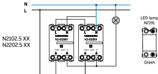
2-way switch - Intermediate switch - 2-way switch
