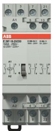
Combination of an installation relay E297 with an attached Contact Module E298-16-11 (additional main contacts) plus an Auxiliary Contact to clearly indicate the switching state of the main contacts (ON/OFF).
