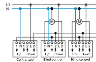
The IR button 8439.XX and the programmer 8165.3 can control a group of blind motors by operating the auxiliary inputs ("1" and "2") of the blind control device. Using a two-pole switch for blinds, the group of blinds can be moved manually or the sensor can be activated for periods of absence.
