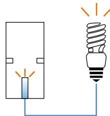
Switches with incorporated LED (see page 2/8) have preinstalled 250V~ LEDs and dedicated terminals for wiring. It is possible to implement any type of functional indication, also with LEDs at different voltages.
