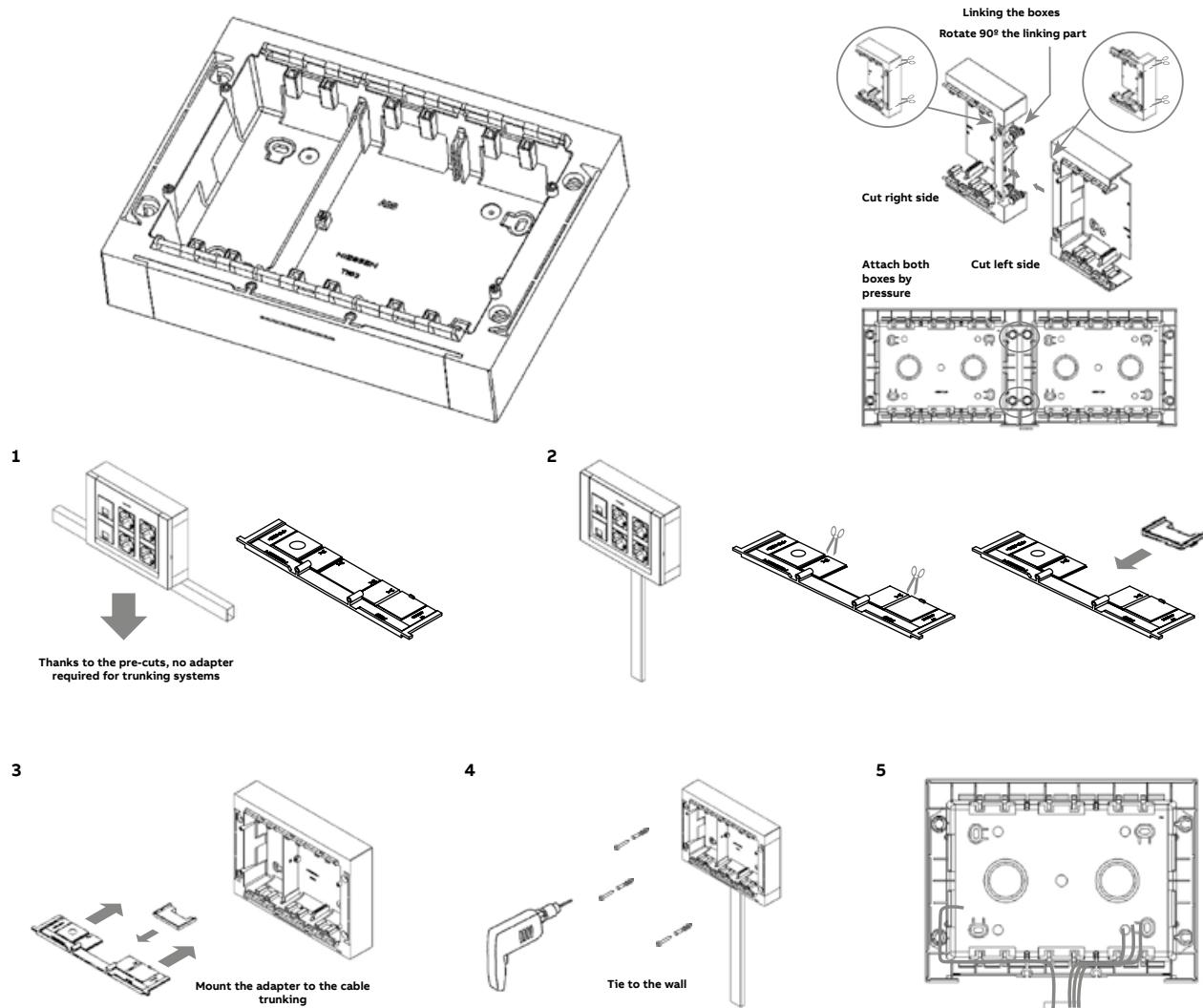
Installation of mechanisms
