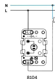
\* The • indicates where the night guide lamp must be connected.
