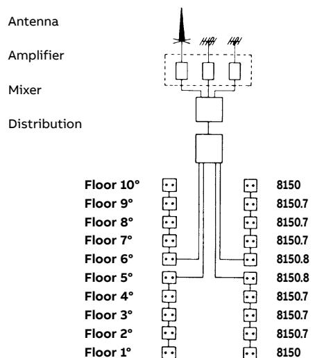
**Example:** 10 floors. The floors are divided in 2 groups of 5 floors each. The outlets are distributed according to the criteria shown in the MATV connection diagram for serial distribution up to 9 floors. The diagram above can be used in buildings up to 18 floors. For buildings with more than 18 floors and up to 27 floors, 3 groups have to be created and so on.
