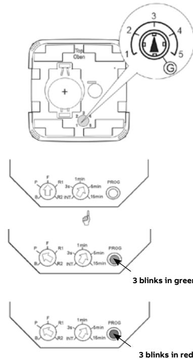
**2.5.-** Place the transmitter and receiver in operation mode:
