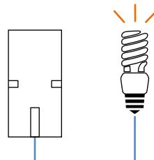
The 2CSY1632MY and 2CSY1633MY LEDs can be added to conventional switches (see page 2/4) for night-time location. The LED electrically connected in parallel with the ON operating mechanism: it is lit when the load is off (OFF command), and it turns off when the load is powered (ON command).
