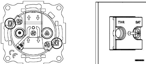
2. There are two options of mounting the cover plates: a) cut the clamps that are facing the small holes.
