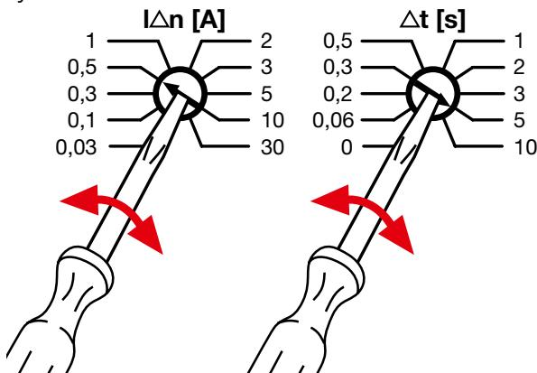
Adjustment of residual operating current ( $\Delta n$  [A]) and trip time delay ( $\Delta t$  [s]).
