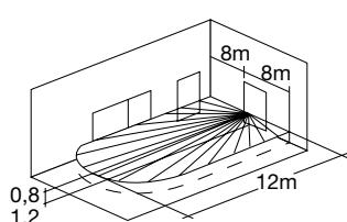
In these applications, the light sources must be outside the detection area to prevent the disconnection due to a Sensor Switch being interpreted as a thermal variation by the other Sensor Switch, causing an unwanted connection.
