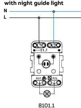
Two-pole switch 16 A with control pilot
