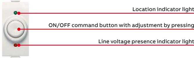
Electronic dimmer with pushbutton control for resistive and inductive loads 60-500W 60-500VA 230V~ -50/60Hz (visible in the dark).
