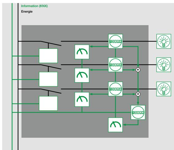
The Energy Actuator facilitates control of the connected consumer loads via the ABB i-bus® KNX. For each of the three switch channels, the individual consumption can be measured in the same way as for the Energy Module. For every channel, the proven functionality of the ABB i-bus® KNX Switch Actuators are available.
