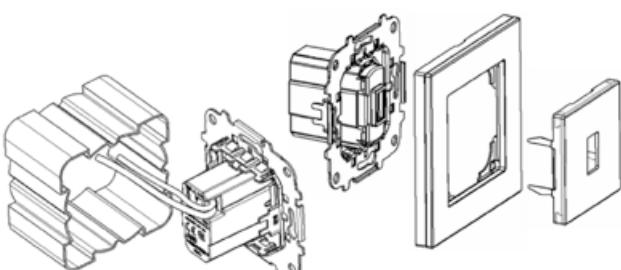
3.3.- Fig. 5. -Installation of USB charger with two outlets 8185.3
