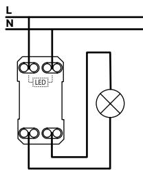
Wiring of double-pole switches 2CSY1006MC/S
