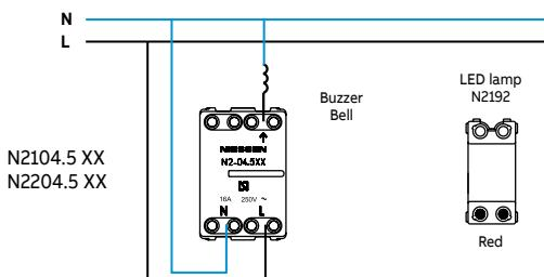
**Push-button for relay with locator lamp**
