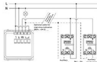
Figure 4: Special wiring diagram
