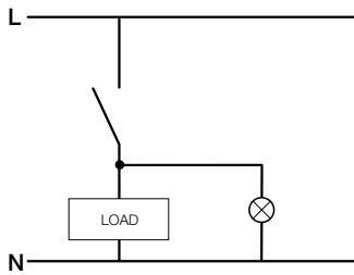
Warning light placed in parallel to the load, of which indicates the ON/OFF state (it is on when the switch is ON).
