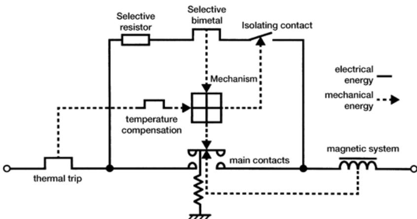
**Functional diagram of selective main circuit breakers S 750 (DR)**
