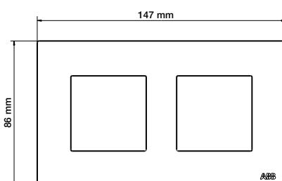
Triple rocker & KNX sensor frame 2 gang
