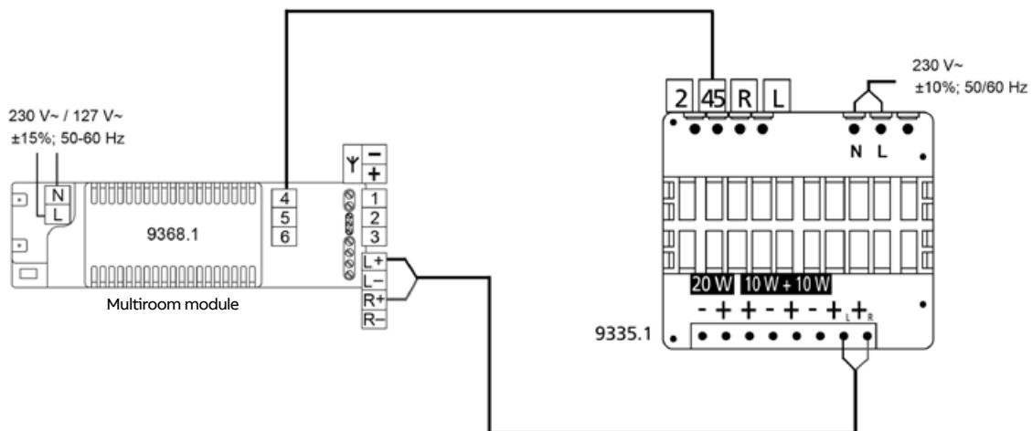
Wiring diagram for 9329.1 loudspeakers to 9335.1 sound amplifier
