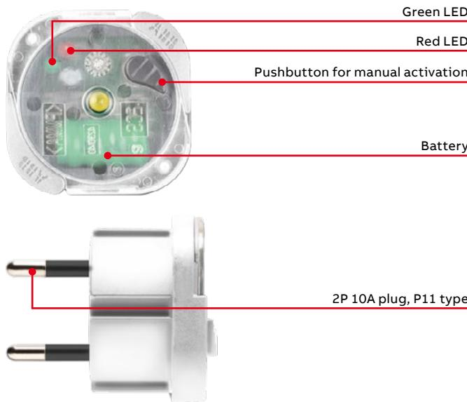
The anti-blackout light is an automatic removable, rechargeable electronic lamp that can be inserted in any Schuko socket or Italian P11 standard 10A bivalent socket. Socket outlets particularly recommended for holding the lamp are the sockets of the Chiara wiring accessories' range 2CSK1108CH and 2CSK1109CH, that allow the body of the lamp to be embedded in the socket outlet, thus minimizing the external dimensions.
