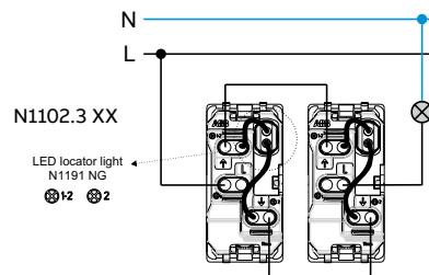
2-way switch - Intermediate switch - 2-way switch
