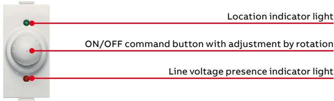
Electronic dimmer with rotary control and two-way switch for resistive loads 100-500W 230V~ -50/60Hz (visible in the dark).
