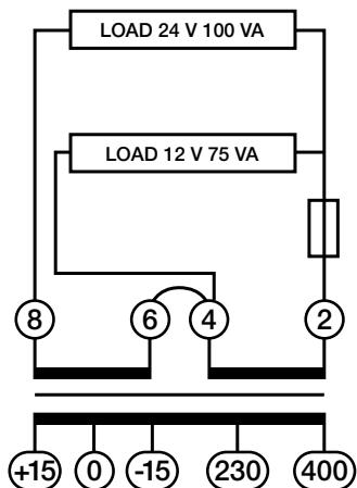
The fuse must be selected based on the higher voltage of the load and positioned in the point where the current of the two loads passes.
