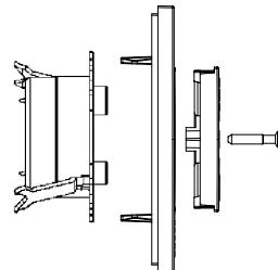
3. When the cover plate is screwed to the insert, the 4 parts that stick out from the cover, will fix the frame to the wall.
