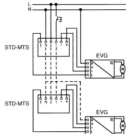
Dimmer STD 50-4 in two-way circuit, lv halogen
