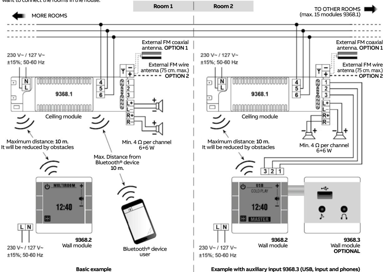
**NOTE:** Because these devices are radio frequency and to avoid interference, you should not install modules of the same reference or any other RF equipment that could interfere less than 1 m. away. It should be noted that any obstacle between the devices, can significantly reduce the distance range between them.
