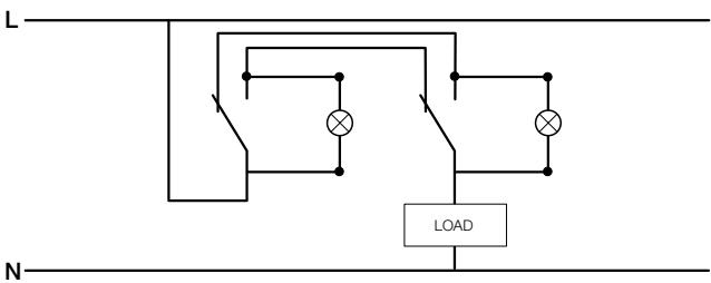
The two warning lights switch on and off respectively when the load is in the OFF and ON state.
