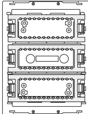
2. Both in the surface solution and in the flush solution, there are metal mounting plates where the mechanisms are inserted.
