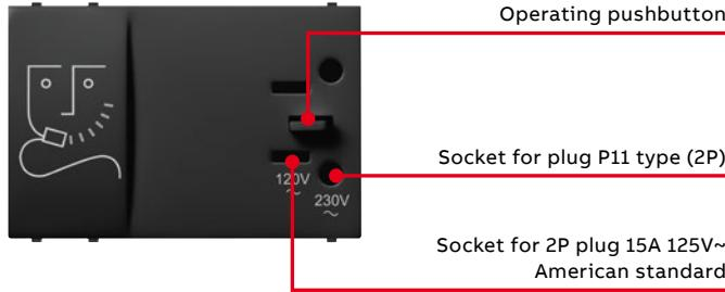
The shaver socket incorporates an insulating transformer with a power rating of 20 VA, protected against overload and resistant to short-circuits.
