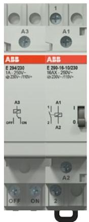
This is a second possibility to implement a Central ON/OFF control. When a E294/... accessory is snapped on, this Central ON/OFF device uses a different voltage source for coil control. The light control can be performed locally on site via the regular button. The Central ON/OFF button permits a general switching state change from a central location.
