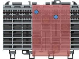
Supply option for auxiliary busbars using incoming terminal block.
