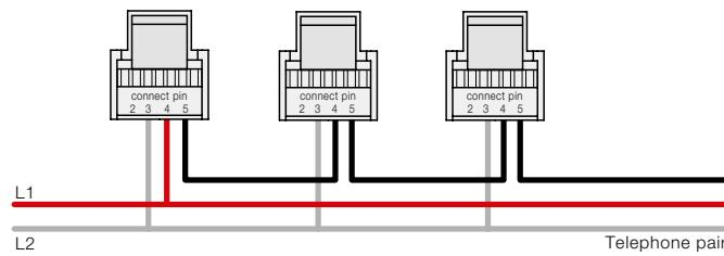
Terminals 3 and 4 are connected via the internal contact to the telephone (closed with the receiver hung up). Lifting the receiver causes interruption of the downstream line (L1), guaranteeing secrecy of the conversation.
