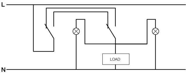
Two warning lights placed in parallel with the load (they switch on and off with it).
