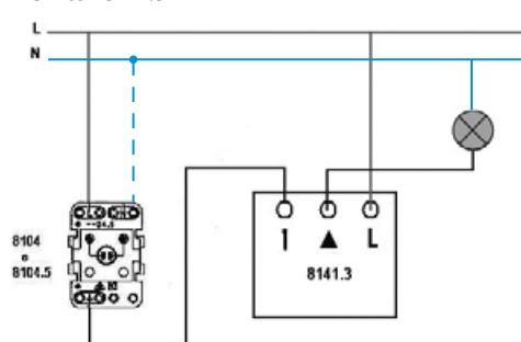
**Note: To use the 8141.3 in parallel, make sure the minimum load is increased by: no. of devices x 60 W**
