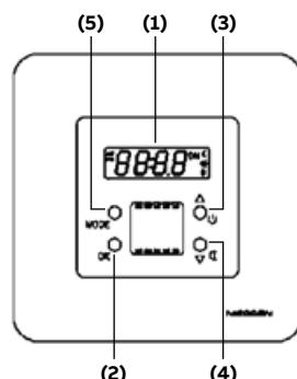
This command allows you to control heating and cooling devices (not simultaneously) from its internal electronic thermostat. Also, thanks to the night mode, allows to maintain a temperature differential (from 0°C to 5°C, also programmable) to save energy with just one keystroke.
