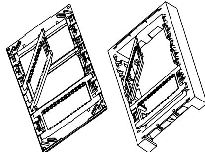
3. The mechanisms are inserted in the mounting plate by pressure.
