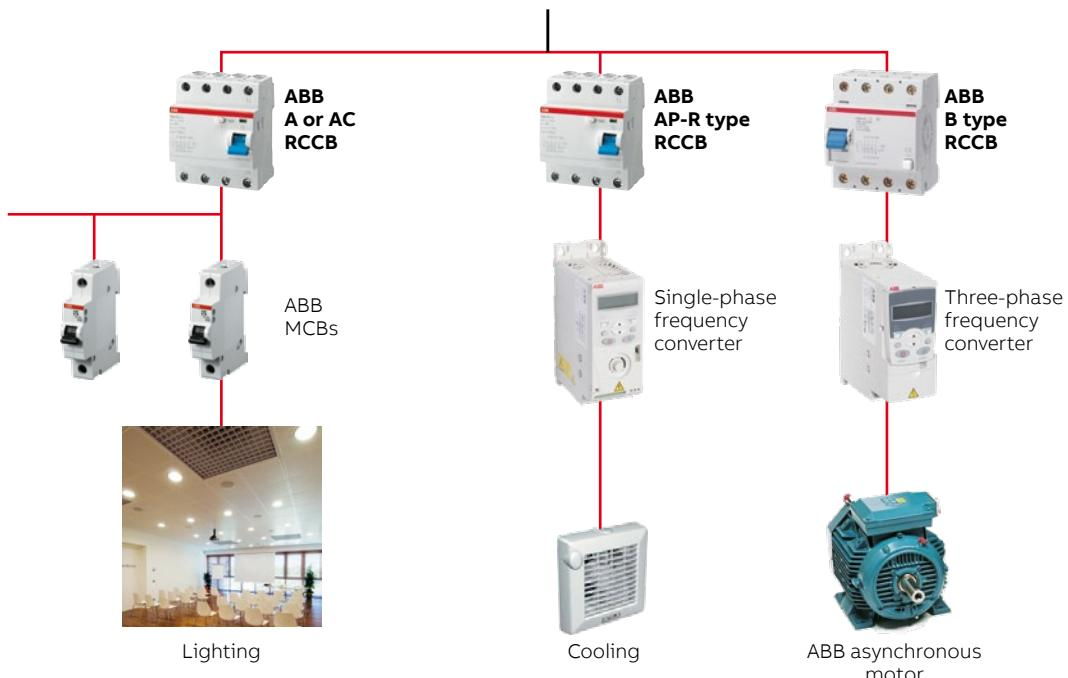
Compared with standard type breakers, AP-R residual current breakers are therefore characterised, for any given sensibility, by:
