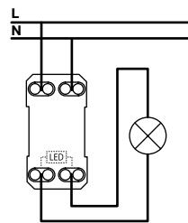
Wiring of double-pole switches 2CSY1006FC/S
