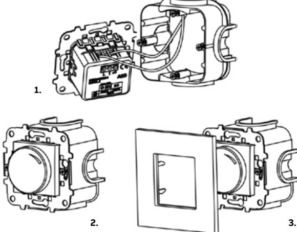
Turn the device in the correct installation position. The marks on the back side of the device, orients the correct top position.
