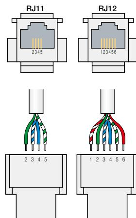
For telephone use, 2 wires of the RJ11 and RJ12 connectors, use the central contacts 3-4
