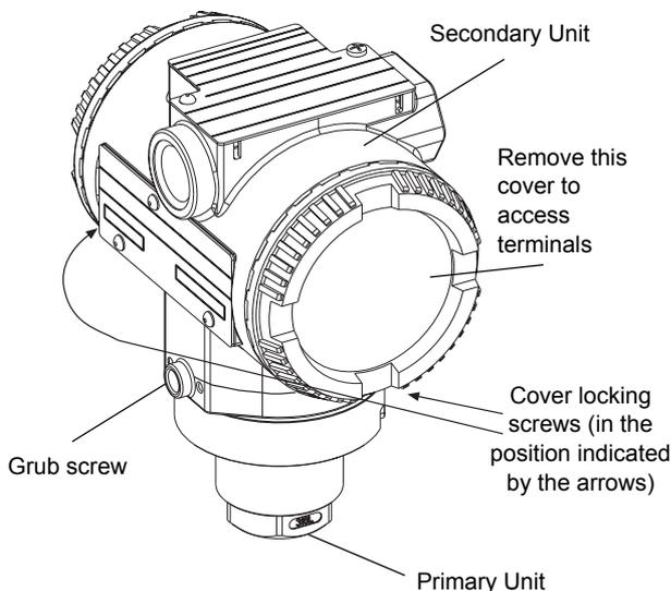
**Fig. 7 - Location of the locking screws and terminals**
