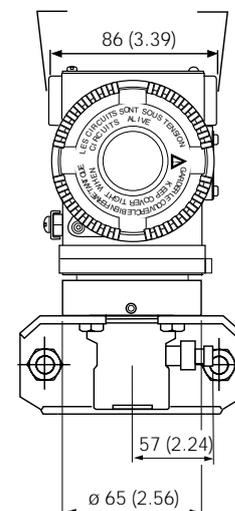
Adapter straight (180°) entry connection (7/16in – 20 UNF drilling)
