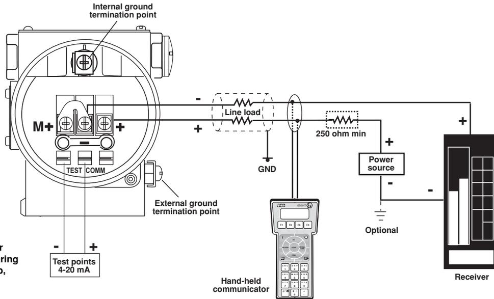
Model 691HT Communicator may be connected at any wiring termination point in the loop, providing the minimum resistance is 250 ohm. If this is less than 250 ohm, additional resistance should be added to allow communications.
