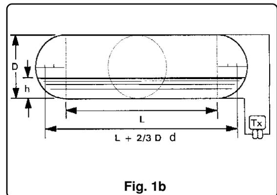
The non conformity error depends on the ratio between diameter and length of the vessel: for ratio  $\geq 5$  to 1 the error is  $\leq 0.25\%$ . The polynomial found with mathematical method gives an error  $\approx 0.15\%$ .
