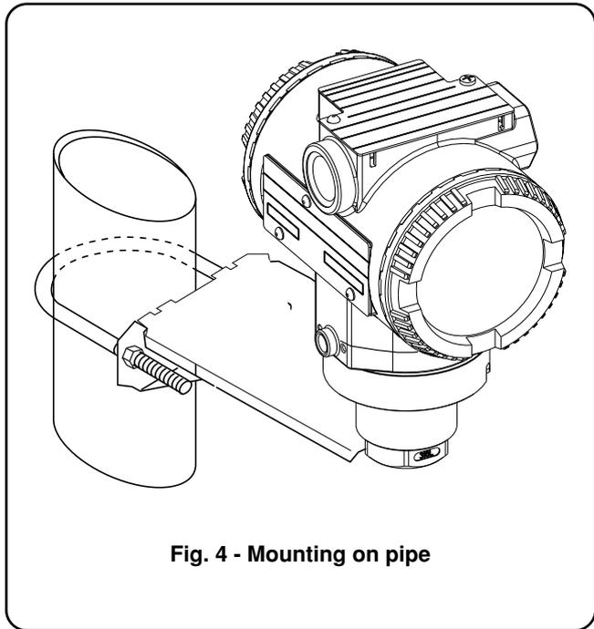
**Fig. 4 - Mounting on pipe**
