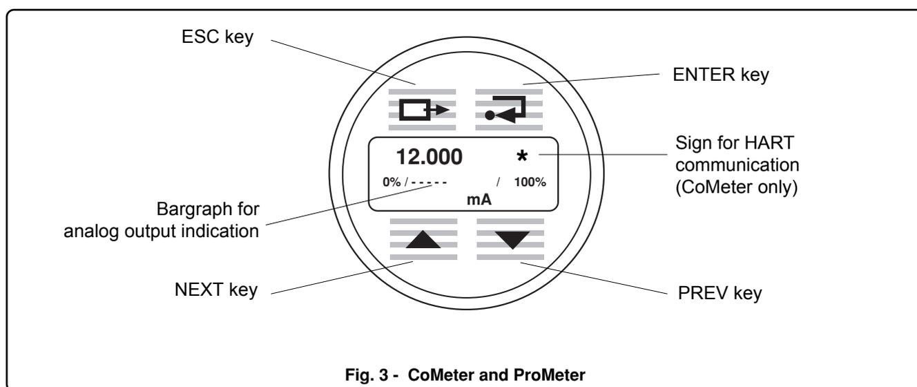
The normal operating condition for CoMeter and ProMeter is to display the analog output signal of the transmitter, expressed in milliAmpere (this is the default setting), or in percentage or in engineering unit, with all the units available as for the HART Communication Protocol.
