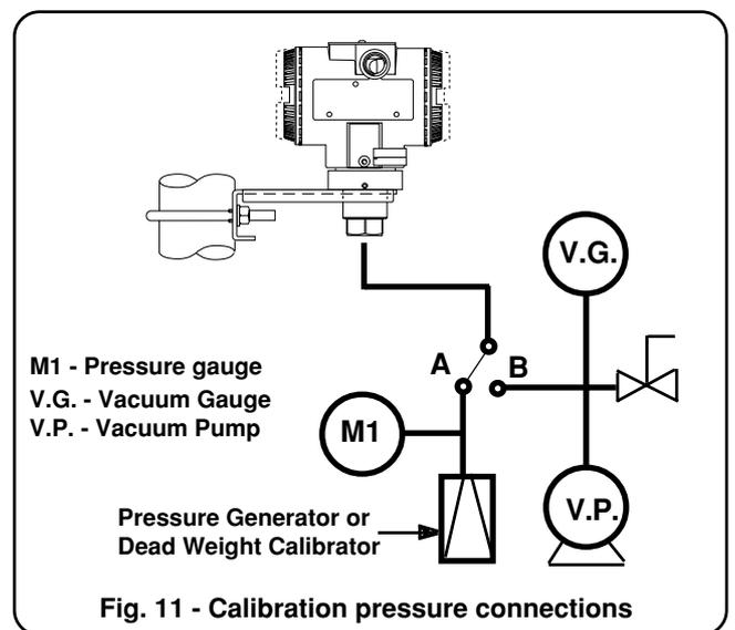
Fig. 11 - Calibration pressure connections
