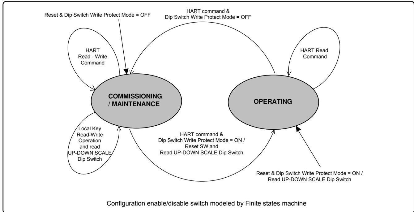
**WARNING** - The transmitter is considered in safety condition (normal operating mode) when the switch is in Write Protect (off). In that condition only reading commands are enabled.
