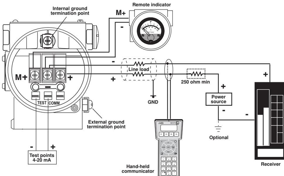
**Fig. 8c - Electrical connections with remote indicator**
