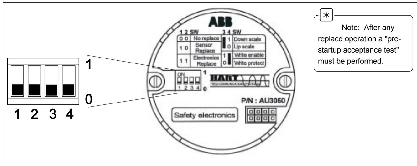
Switches 1 and 2 are used for Electronics or Transducer replace; Switch 3 is for Write Protect mode selection; Switch 4 is for Up/Down Scale selection. Here below a description of the operations.
