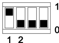
Switch 1 up in "1" position is required before power up the transmitter, when a replace is being performed. Switch 2 down in "0" position allows the replace of the transducer.
