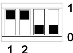
Switch 2 up in "1" position allows the replace of the secondary electronics. It must be moved in this position, when electronics replace is being performed, before power up the transmitter.
