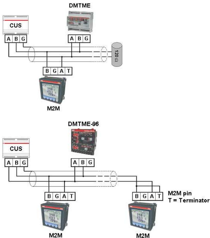
In the previous figure, if the M2M is the last instrument installed in the RS485 network, is possible to avoid the terminal resistor connecting pin T with pin B.
