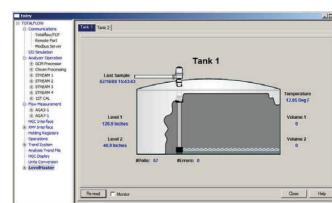
shows the levels, volumes, temperature, timestamp of last data sample and if any error codes are present. You can quickly view each tank by selecting the appropriate tab at the top of the window.
