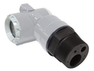
The SS140XP level sensor is certified for use in hazardous areas in North America and Russia (FM, CSA and GOST-R approvals). ABB has identified an issue with the design of the SS140XP that can cause the front lens on the device to crack in certain instances when it is subjected to high temperature (above 50°C) thermal cycling. Once the lens cracks, there is potential of compromising the flame proofed enclosure which may invalidate the hazardous area protection.
