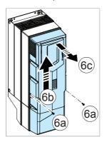
Install the hood to UL Type 12 drives after you have installed the drive electrically and reinstalled covers, refer to Installing UL Type 12 hood (page 232).
