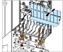
15. Ground the motor cable shield at the motor end. For minimum radio frequency interference, ground the motor cable shield 360° at the cable entry of the motor terminal box.
