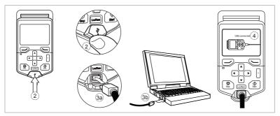
Alternatively, you can connect an Ethernet networking cable (eg. Cat 5e) to the Ethernet port behind the control panel. Make sure that the control panel is placed on a platform or a DIN rail.
