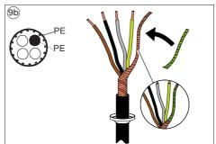
10. Connect the input power cable. Use terminals L1, L2 and L3. Tighten the screws to the torque given in the table.
