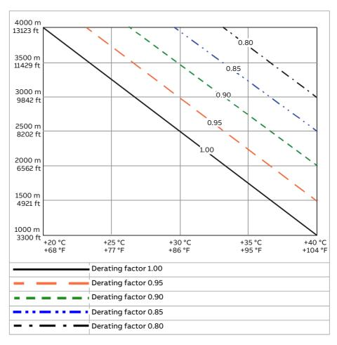
**Note:** Check the supply network compatibility restrictions above 2000 m (6562 ft), see **Installation site altitude** (page 379). Check also PELV limitation on relay output terminals above 2000 m (6562 ft), see sections Isolation areas (page 250) for frames R1...R5 and Isolation areas (page 254) for frames R6...R9.
