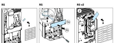
4. Remove the rubber grommets for the motor and input power cables, as well as brake resistor cable, if used.
