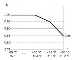
$\underline{-260A-4, -293A-4; -273A-2, -276A-2}$ : In the temperature range +40...45 °C (+104...113 °F), the rated output current is derated by 1% for every added 1 °C (1.8 °F). In the temperature range +45...50 °C (+113...122 °F), the rated output current is derated by 2.5% for every added 1 °C (1.8 °F). The output current can be
