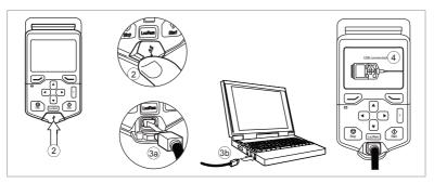
Alternatively, you can connect an Ethernet networking cable (eg. Cat 5e) to the Ethernet port behind the control panel. Make sure that the control panel is placed on a platform or a DIN rail.
