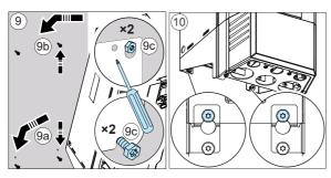
Install the hood to UL Type 12 drives after you have installed the drive electrically and reinstalled covers, refer to Installing UL Type 12 hood (page 232).
