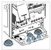
**Note:** The drive is shipped with grommet cones pointing up. They must be removed and inserted back pointing down.
