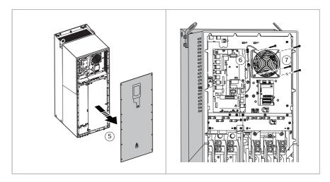
8. Install the new fan in reverse order, tightening torque of the fan screws 0.5 Nm.
