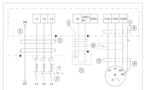
**Note:** UL (NEC) installation can include separate insulated conductors inside a conduit, shielded VFD cable in conduit, or shielded VFD cable without conduit. The normal dashed symbol (3) in this diagram represents the shield of shielded VFD cable. The same solid symbol (2) represents conduit.
