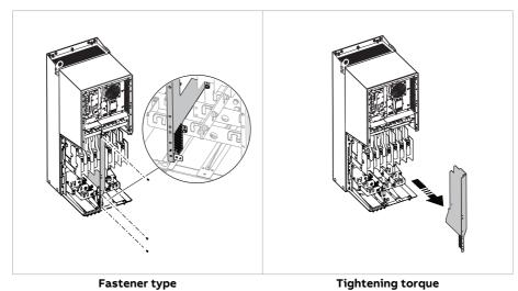
Remove the control cable entry plate
