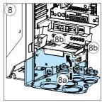
Install the hood to UL Type 12 drives after you have installed the drive electrically and reinstalled covers, refer to Installing UL Type 12 hood (page 232).
