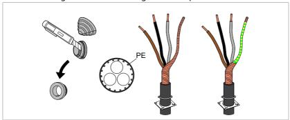
e. Cut off one phase conductor from the DC cable.
