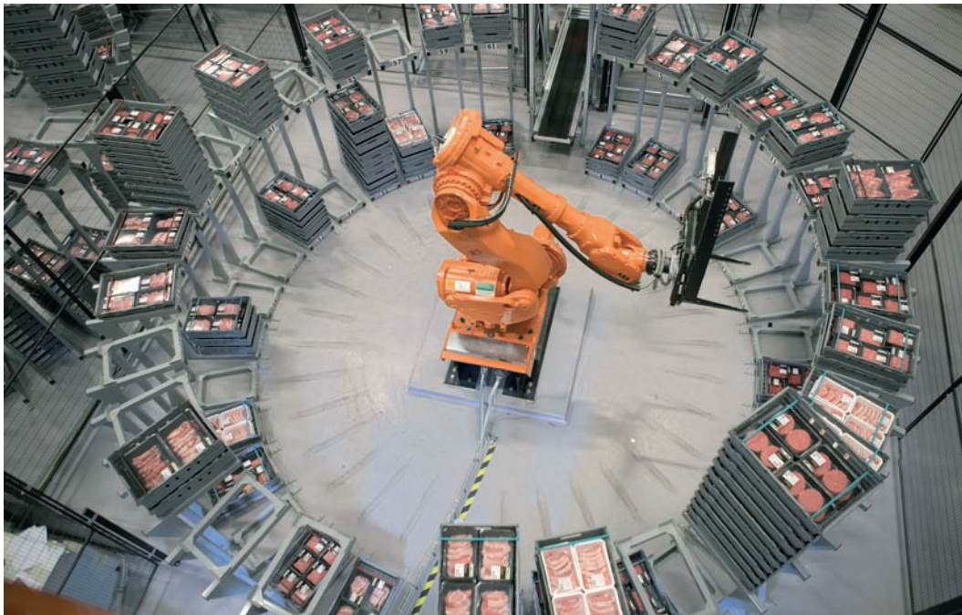
A single robot is used to organize small quantities of inventory to efficiently stage individual orders to be shipped
