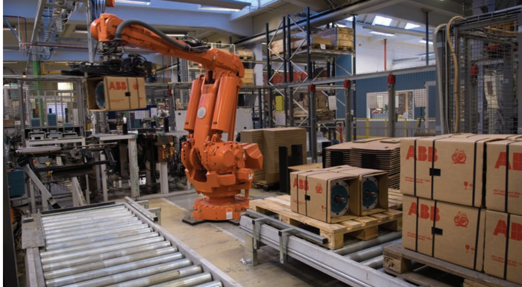
Robots speed the palletizing of motors while reducing waste, and the concern of a worker being hurt
