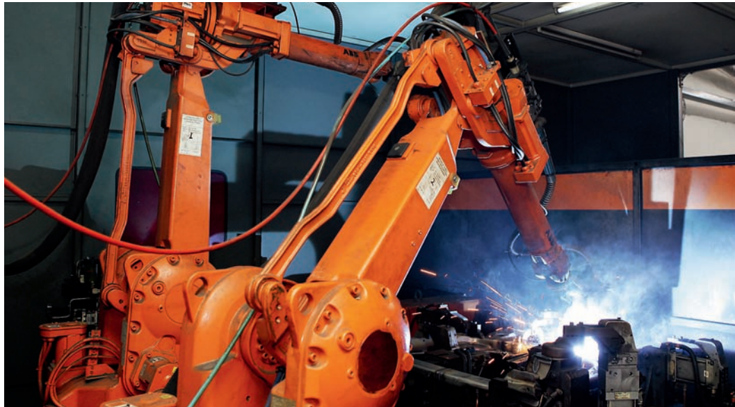
Two robots are used to load, unload and weld parts with little human intervention and with a high degree of accuracy
