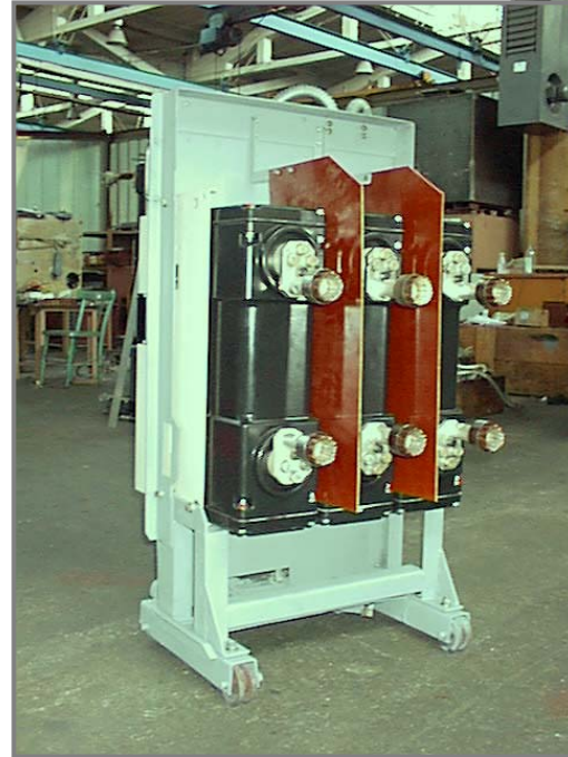
Retrofit of Russian switchgear by replacing the oil- minimum breaker with SF 6 circuit breaker type HPA
