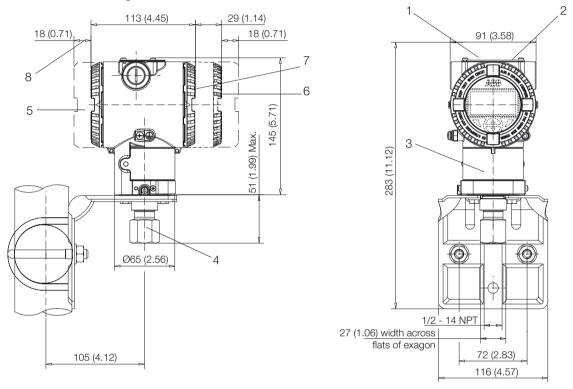
1 Adjustments | 2 Identification plate | 3 Certification plate | 4 Process connection | 5 Terminal side | 6 Integral display housing | 7 Electronic side | 8 Space for cover removal
