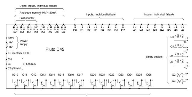
Failsafe inputs / Outputs (not failsafe) / Dynamic outputs
