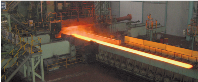
Zhangjiagang Hongchang's plate mill, producing 5 meter wide plates
