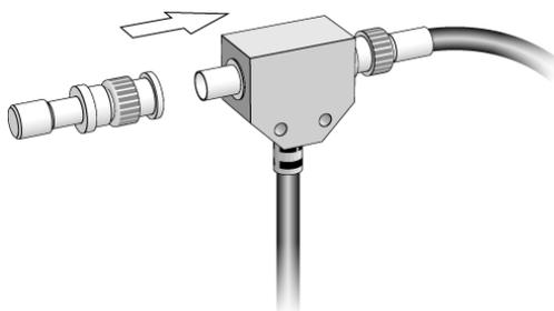
Figure 70. Install a 75Ω terminator onto the tap's other BNC connector.
