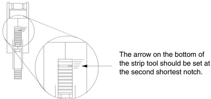
Figure 45. Stripping the cable, step 1.
