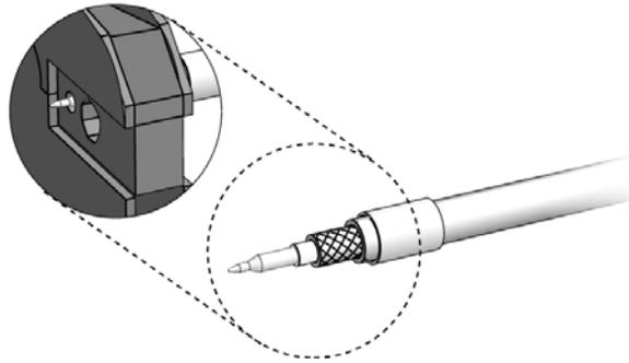
*Figure 59. The smaller hexagonal crimping notch is for crimping the center pin onto the center connector.*
