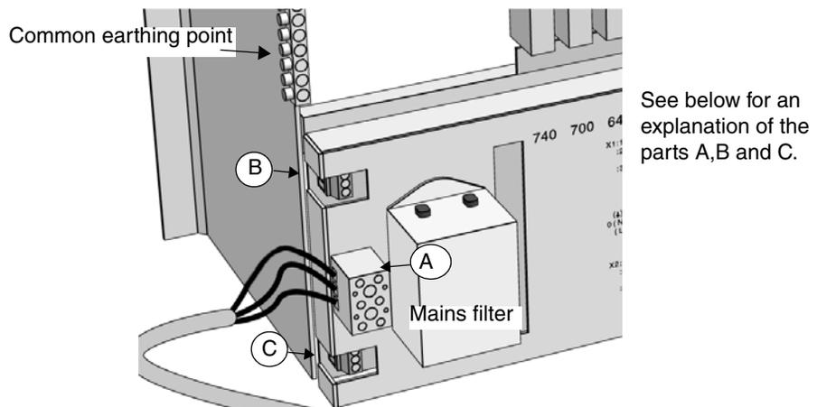
*Figure 24. The mains supply connection.*
