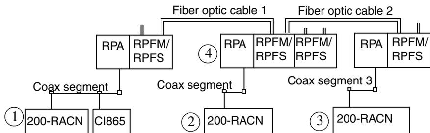
Figure 90. Installing fiber repeaters, example 2
