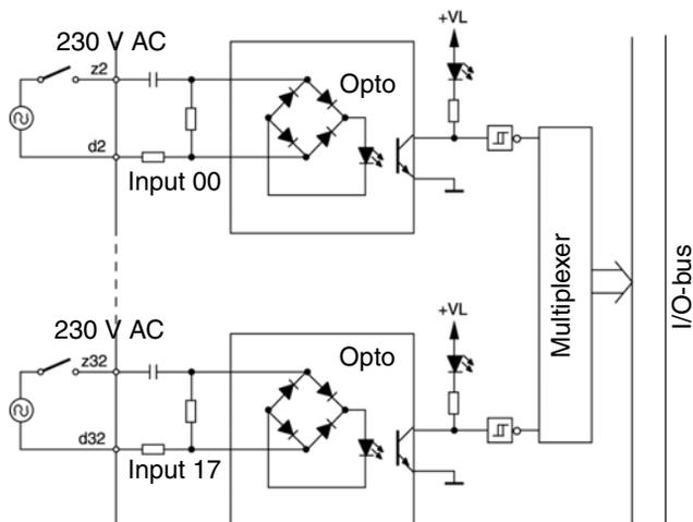
Figure 96. Block diagram IAPG230. The d-pins can be tied together if a neutral reference is required.
