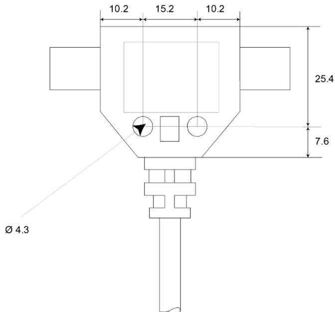
Figure 121. Mounting Dimensions, T-tap
