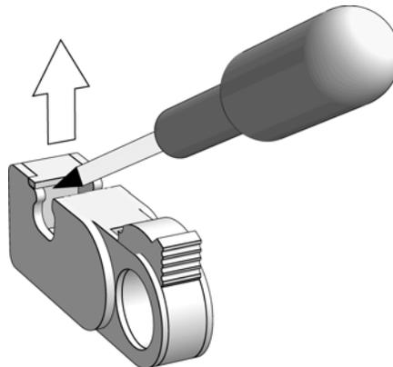
Figure 129. Lifting the memory blade holder.
