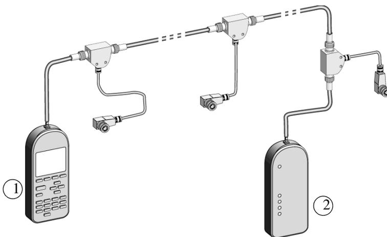
Figure 66. Example of a TDR with main unit (1) and remote unit (2).
