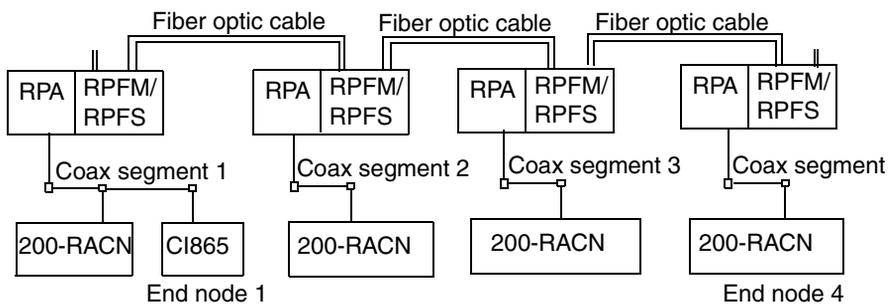
Figure 89. Installing fiber repeaters, example 1
