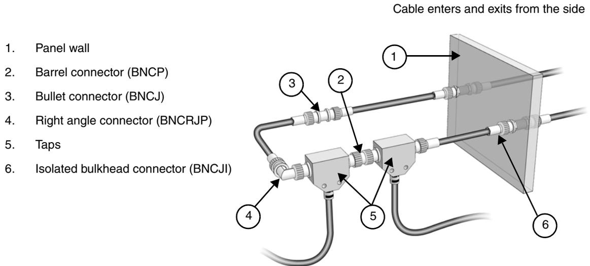
Figure 34. Example of how to use different connectors.
