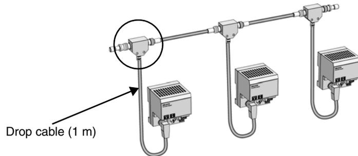
Figure 5. Tap connections via drop cable.
