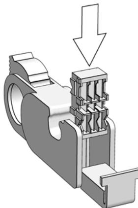
*Figure 132. Replacing the memory blade cartridge.*
