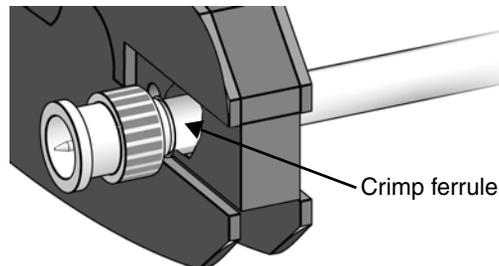
Figure 63. The larger hexagonal crimping notch is for crimping the ferrule which holds the connector to the cable.
