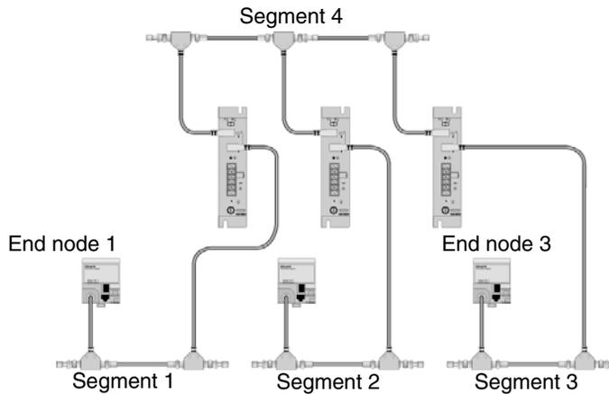
Figure 79. Installing coax repeaters, example 2.
