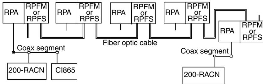
Figure 36. Connection of two coax segments by a chain of fiber repeaters.
