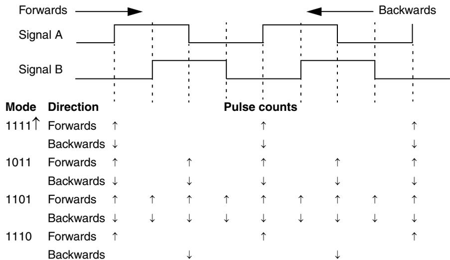
The evaluation logic can be schematically described as in the table below:
