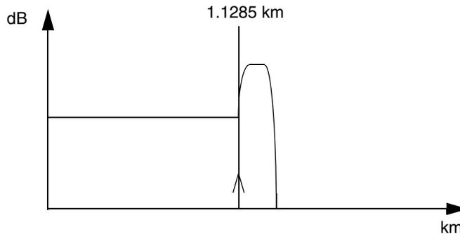
Figure 82. Trace with the marker indicating the total cable length.
