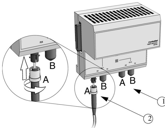
*Figure 87. Fiber channels (1) and (2), receive connectors (A) and transmit connectors (B).*
