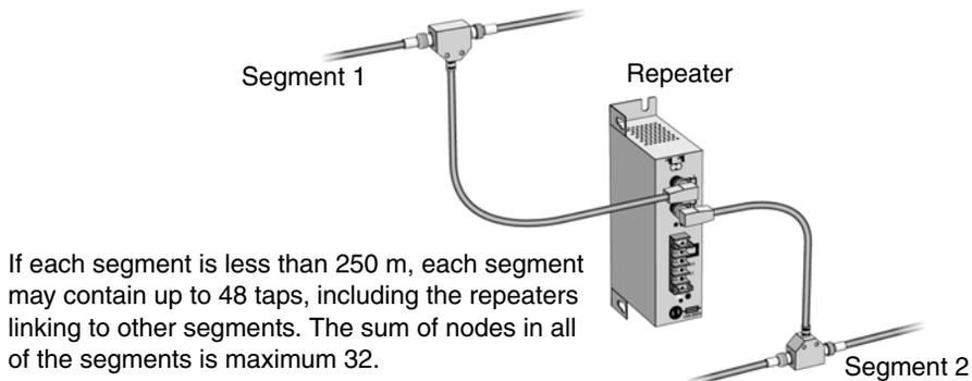
Figure 33. Determining whether repeaters are needed
