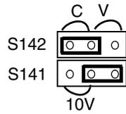
Figure 110. 4-20 mA on channel 14
