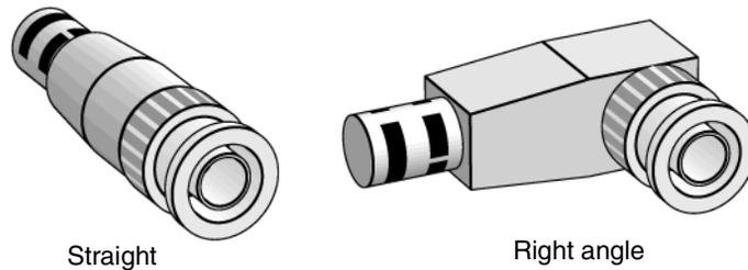
*Figure 7. Taps with a straight or right angle connector on the drop cable.*
