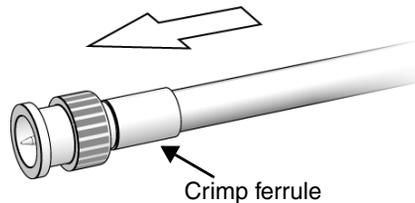
Figure 62. Slide the crimp ferrule into place.
