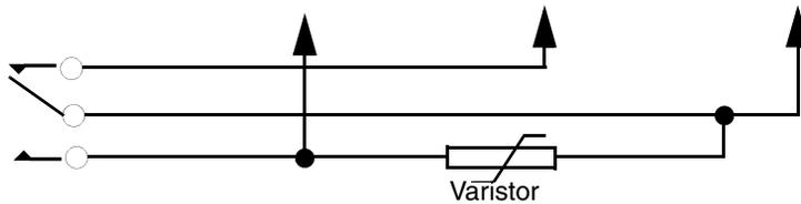
Figure 99. Scheme for X1 connector
