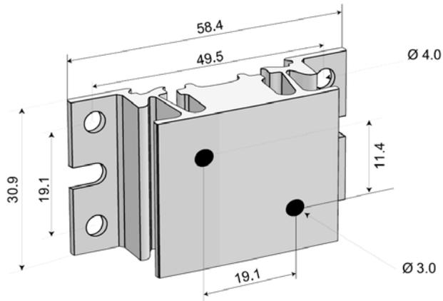
Figure 123. Mounting Dimensions, Universal Mounting Bracket
