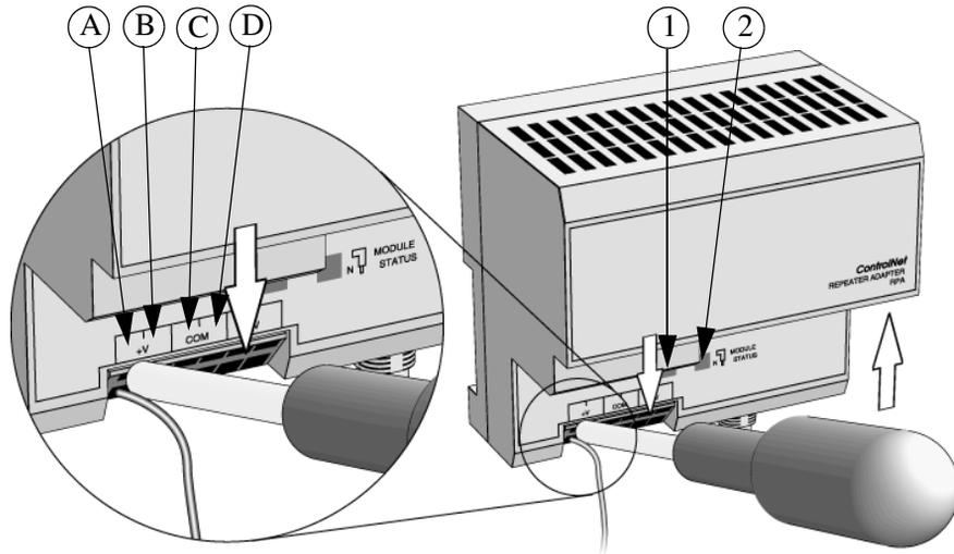
Figure 86. Power terminals A-D, and indications for coax connector (1) and fiber channels (2).
