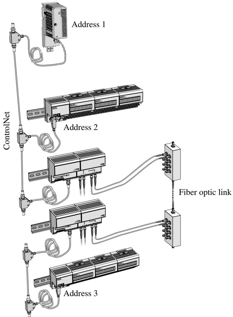
Figure 20. Series 200 I/O connected to ControlNet
