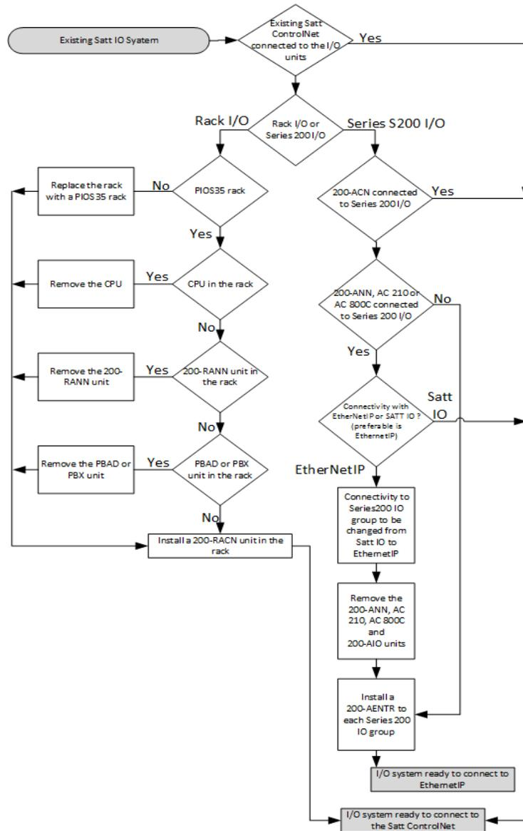
Figure 22. Graphic representation of the rebuilding process.
