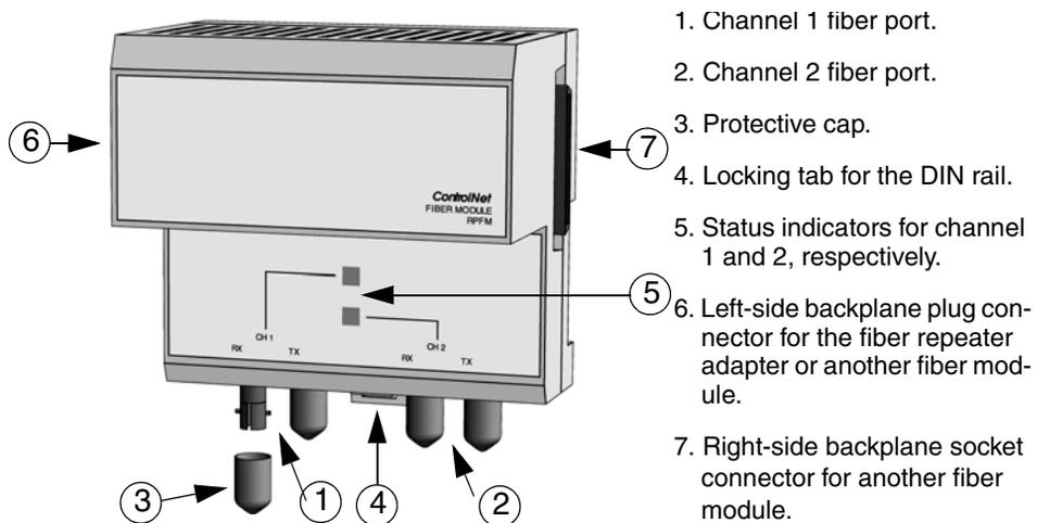
*Figure 15. Fiber Module RPFM and RPFS*
