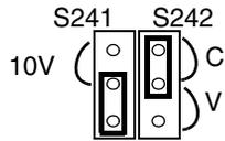
Figure 109. 0-20 mA on channel 24
