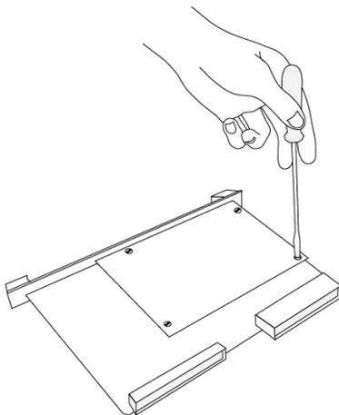
*Figure 114. Removing the insulation plate.*
