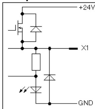
Figure 101. Connector X1 pin assignment and output block diagram ODSG.
