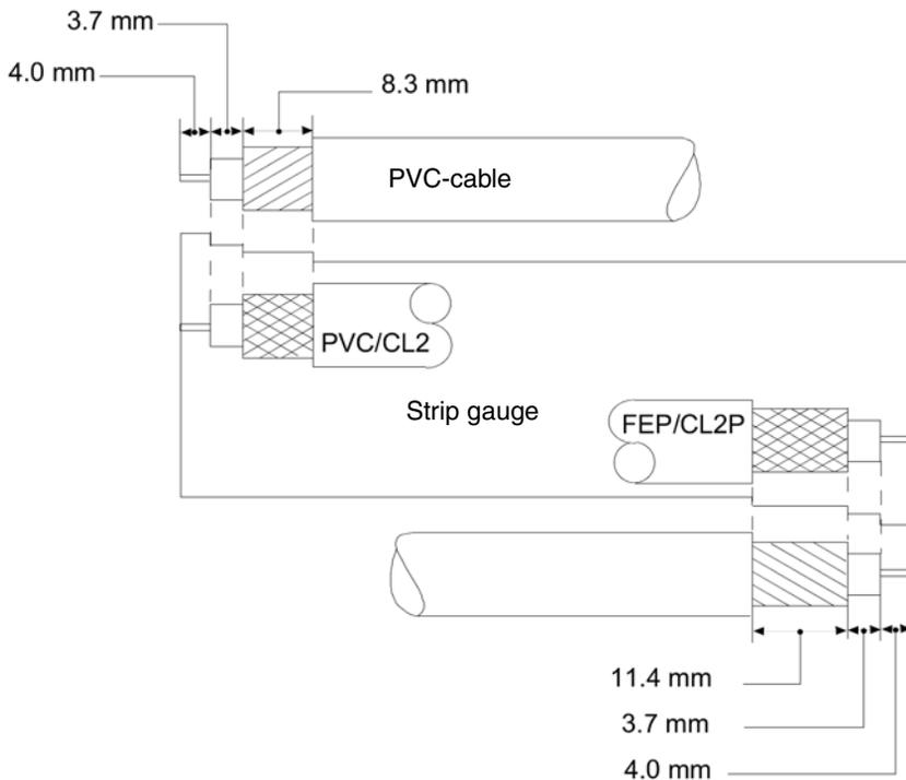
Figure 54. Template for PVC and plenum FEP cable.
