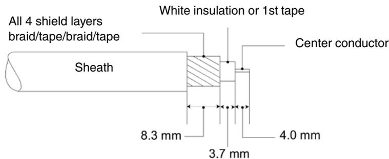
Figure 51. The layers of the cable.
