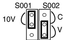
Figure 111. 0-10 V on channel 00
