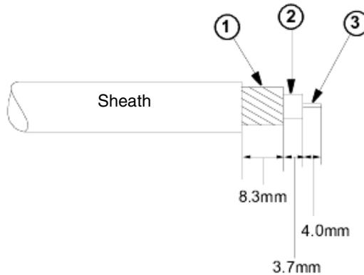
Figure 128. Stripped cable; layers and dimensions.
