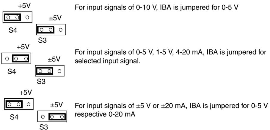
Figure 112. Note that the 0-10 V setting on the IBA is not used.
