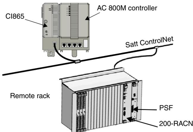
Figure 18. Rack-based I/O system connection alternative.
