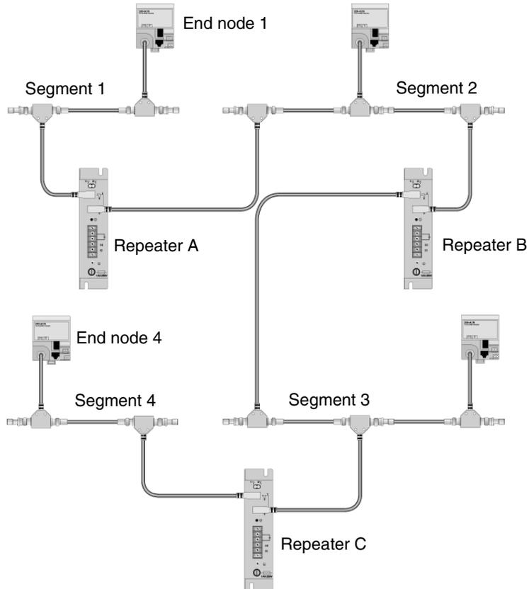
Figure 78. Installing coax repeaters, example 1.
