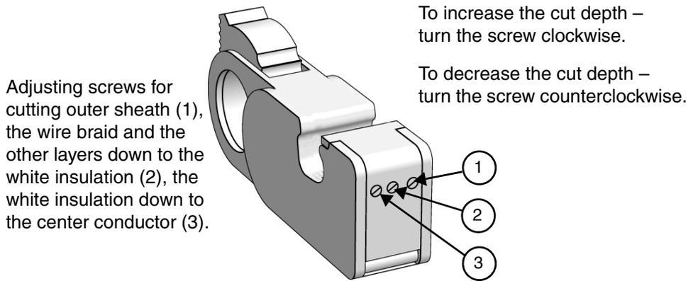
Figure 127. Cable strip tool, adjusting the cutting blades.
