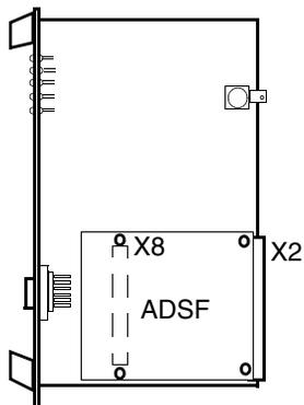
*Figure 93. ADSF - analog-to-digital converter mounted on rack adapter board, 200-RACN.*
