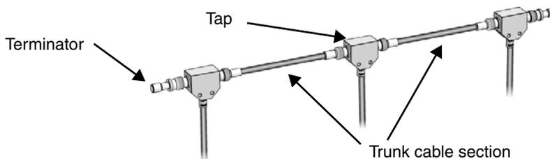
*Figure 30. Determining trunk cable section lengths*
