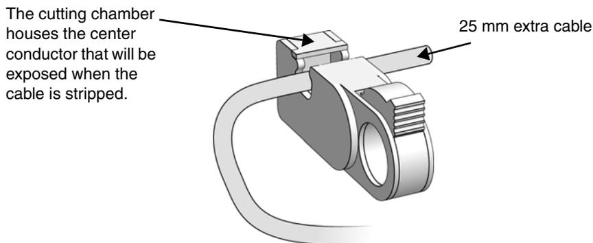
Figure 47. Stripping the cable, step 3.
