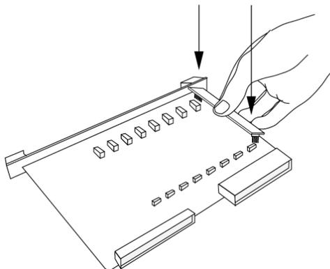
*Figure 115. Fitting the module to the IBA board.*
