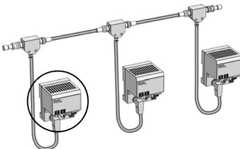
*Figure 4. Example of a node is the ControlNet adapter 200-ACN. Refer to the S200 I/O, Hardware and Installation, User's Guide (3BSE021356Rxxxx) for information about 200-ACN.*
