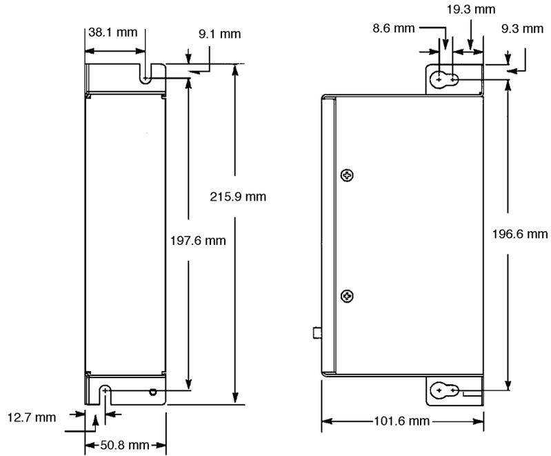
*Figure 124. Mounting Dimensions, Coax Repeater*
