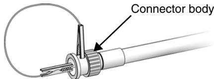
If the resistance readings indicate that there is no short – use your wire cutters to cut off the connector, install a new connector and begin testing again.
