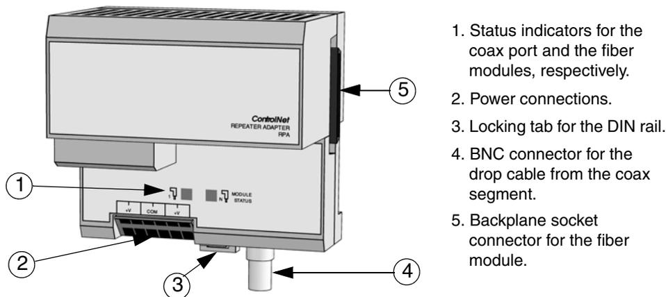
Figure 14. Fiber Repeater Adapter RPA
