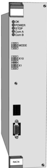
The rack adapter board, 200-RACN, handles the communication between system AC 800M and the remote rack-based I/O system via ControlNet.
