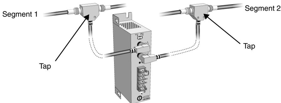
Figure 77. Connect the second tap to the repeater
