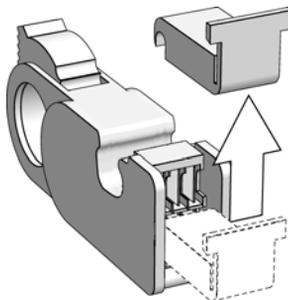
*Figure 135. Removing the memory blade holder.*
