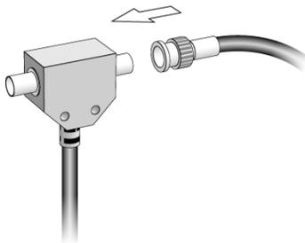
Figure 69. Connect one end of the trunk cable section to one of the tap's BNC connectors.
