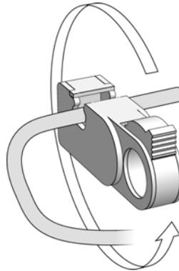
*Figure 49. Stripping the cable, step 5.*
