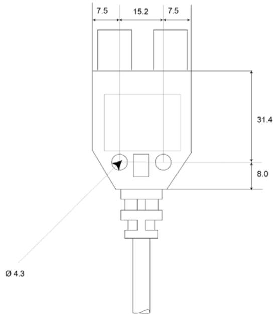
Figure 122. Mounting Dimensions, Y-tap
