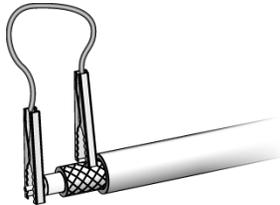
If the resistance readings indicate that there is no short circuit – replace the trunk cable section.
