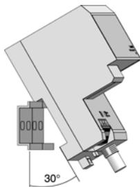
Figure 83. Installing ControlNet fiber units, step 1.
