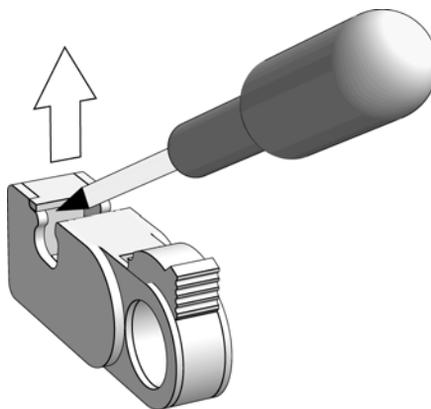
*Figure 134. Lifting the memory blade holder.*
