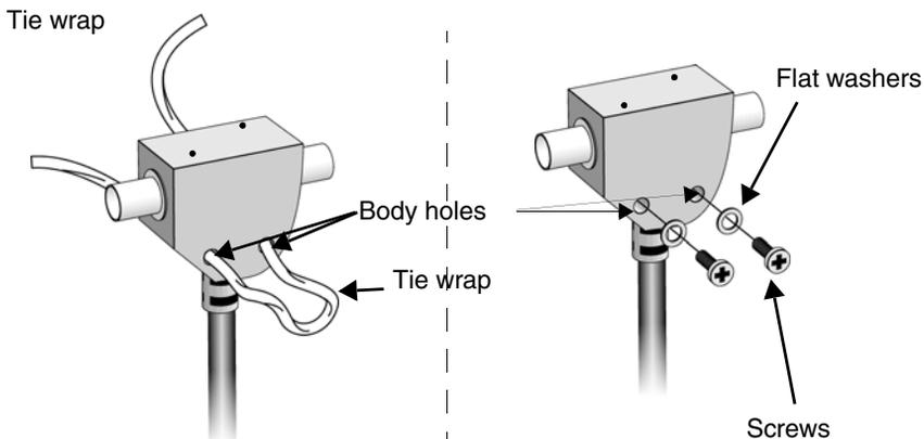
Figure 43. Mounting a tap through the body holes.
