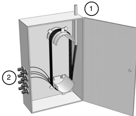
Figure 38. Connector panel with incoming multi-fiber backbone cable (1) and connectors for interconnect cables (2).
