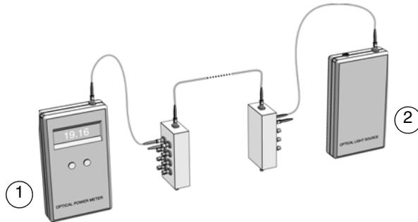
Figure 80. Power meter (1) and 1300 nm light source (2).
