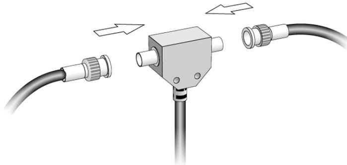
Figure 68. Connecting cable sections
