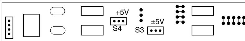
Figure 113. Locations of jumpers S3 and S4 on the MCV200.
