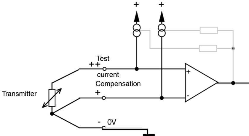
Figure 116. Connecting a temperature or resistance transmitter.
