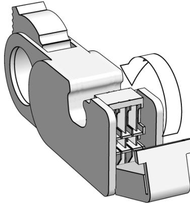
*Figure 136. Closing the memory blade holder.*
