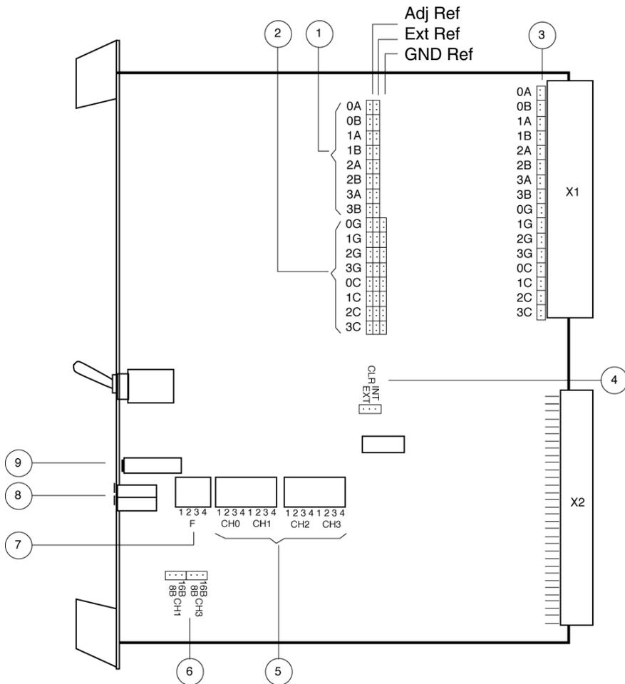
Figure 105. Location of jumpers and DIP switches
