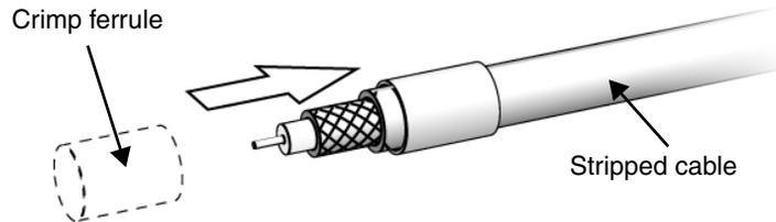
Figure 57. Slip the crimp ferrule onto the cable.
