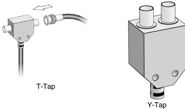
Figure 6. Taps with T or Y placement of BNC connectors.
