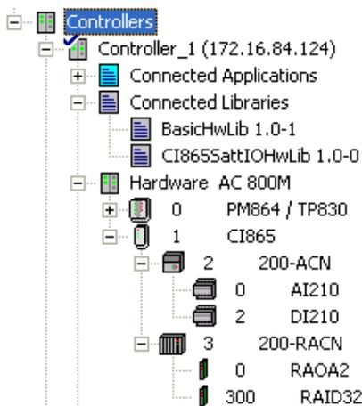
Figure 40. Example of hardware connected to the Satt ControlNet.
