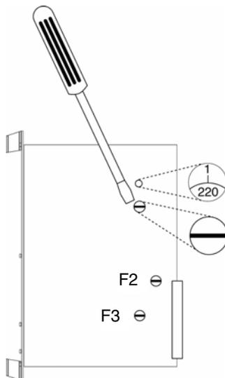
Figure 94. PSF mains supply selection.
