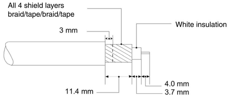
Figure 52. The layers of the FEP cable.
