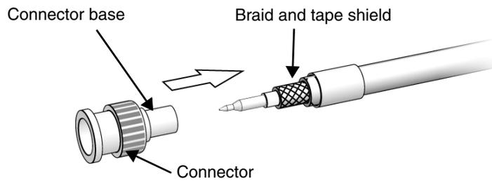
*Figure 60. Slide the ControlNet connector onto the cable.*
