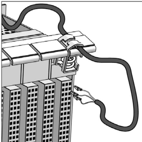
Figure 25. A shielded cable where the shield is grounded with a spring clamp. Crimp sleeves are crimped to the three wires of the cable.
