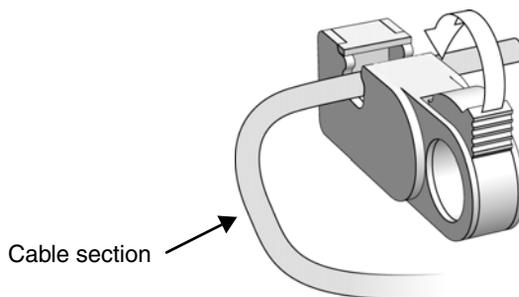
Figure 48. Stripping the cable, step 4.
