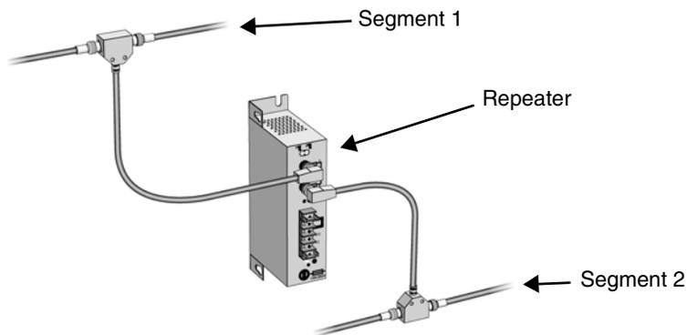
*Figure 13. Segments Connected with a Repeater*
