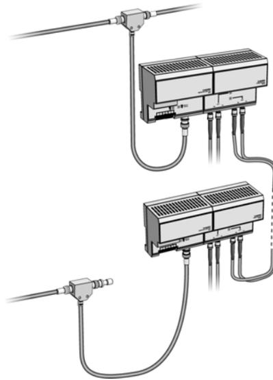
*Figure 35. Two coax segments connected point-to-point.*
