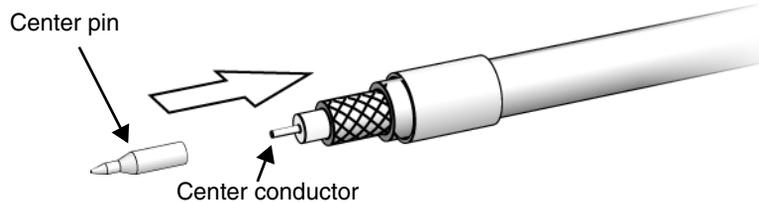
Figure 58. Place the center pin over the center conductor.
