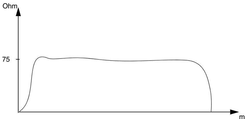
*Figure 67. Normal trace of the relative impedance along a single trunk cable section.*
