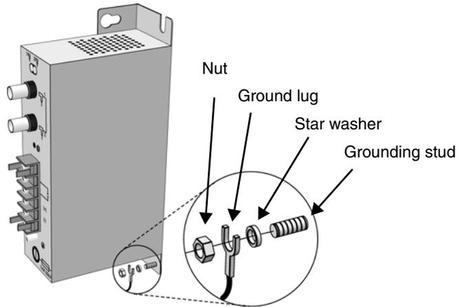
*Figure 71. Ground the repeater*
