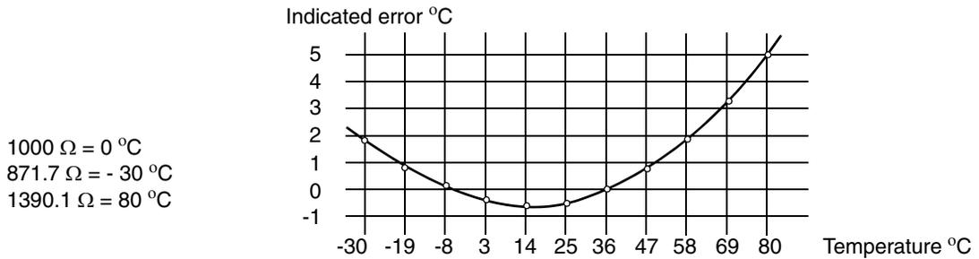
Figure 126. Temperature diagram for MN80.
