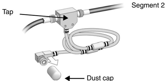
Figure 76. Remove the dust cap from the connector for segment 2.
