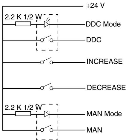
Figure 119. Example of manual control connection.
