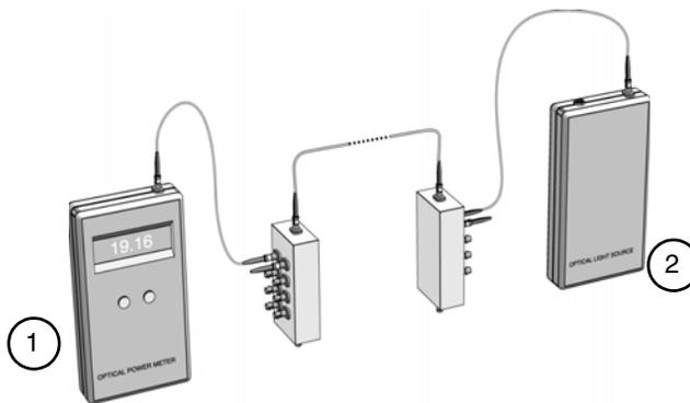
Figure 39. Power meter (1) and 1300 nm light source (2).
