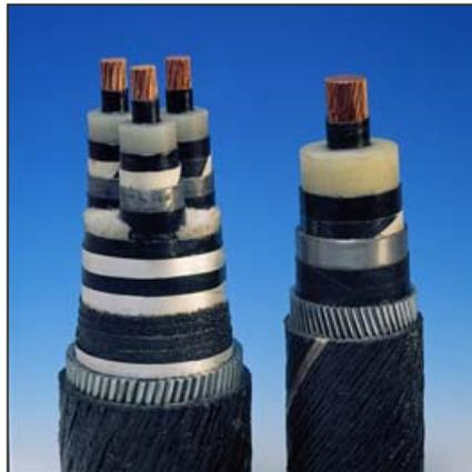
The 110 kV cables were supplied with 300 mm<sup>2</sup> and 400 mm<sup>2</sup> copper conductors respectively. Both cables have a triple-extruded 15.5 mm thick XLPE insulation and a lead sheath protected by a PE jacket. Again, swelling-powder in the conductor and swelling-tapes below the lead sheath further protect the cable from water penetration. The cables also have continuous aluminium-wire armour with an outer protection of bitumen-bonded polypropylene yarn.
