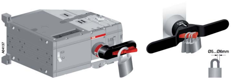
Figure 3.4 Locking the manual operation
