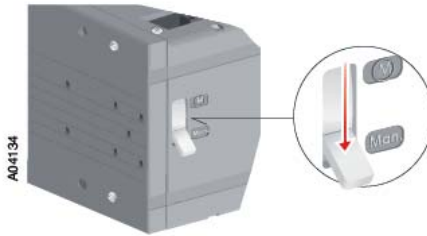
Figure 6.5 Motor/Manual selection in the Man. position
