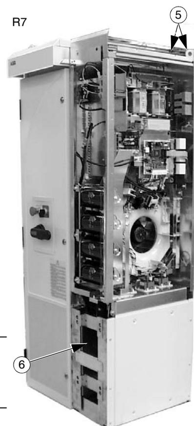
7. The following cables between the drive and the extension module are split by a connector located at the front of the drive. Disconnect both cables at this location.
