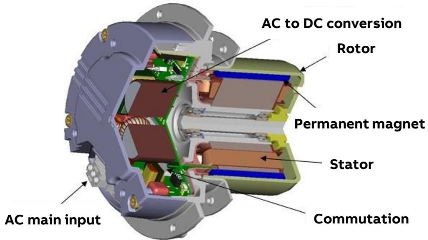
EC motors have an AC/DC conversion with a rectifier built-in
