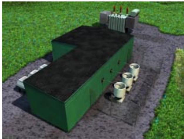
Fig.15 : Typical SVC Light for utility applications.
