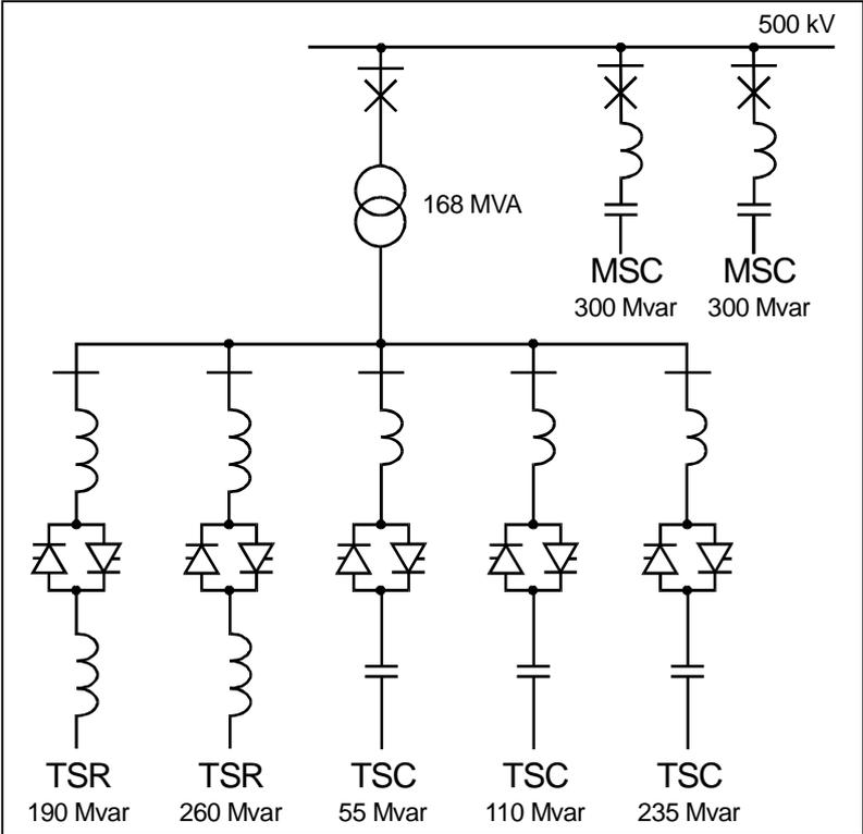
Fig. 7: Single-Line Diagram of the SVC
