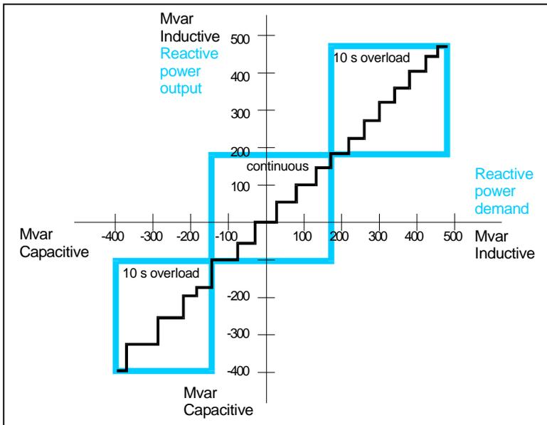
Fig. 8: Dynamic Operating Characteristics of the SVC
