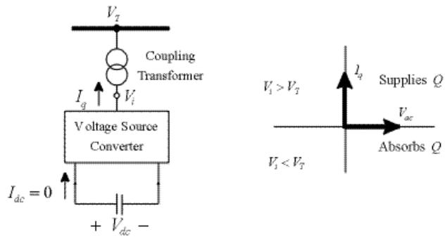
Fig.14 : Static Compensator.
