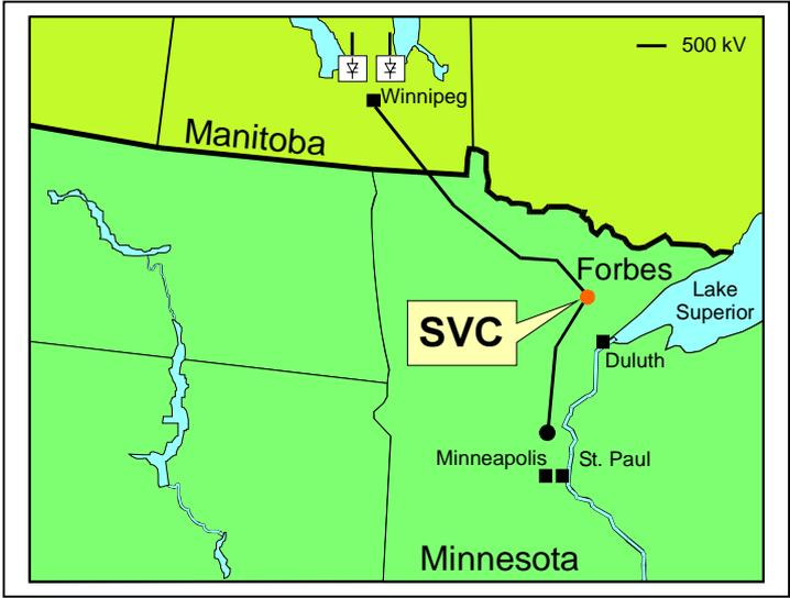
Fig. 6 : Manitoba – Minnesota 500 kV Interconnection
