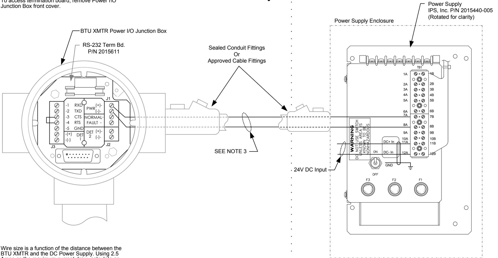
3. Wire size is a function of the distance between the BTU XMTR and the DC Power Supply. Using 2.5 Amps as the maximum current draw, calculate an adequate wire size so that the voltage measured at the BTU XMTR's Power I/O Junction Box is a minimum of 12.5 Volts.
