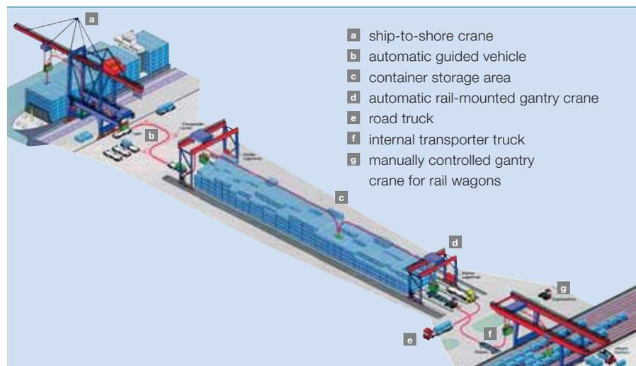
**2** With modern ship-to-shore cranes a ship with 4000-5000 TEU (twenty feet equivalent) to unload/load can be handled in less than 24 hours
