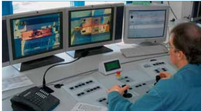
**5** The load positioning system uses infrared sensors to identify the precise load position
