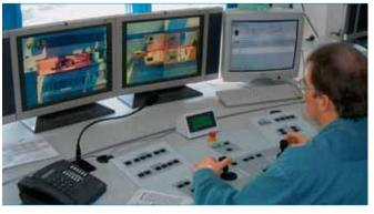
The load positioning system uses infrared sensors to identify the precise load position
