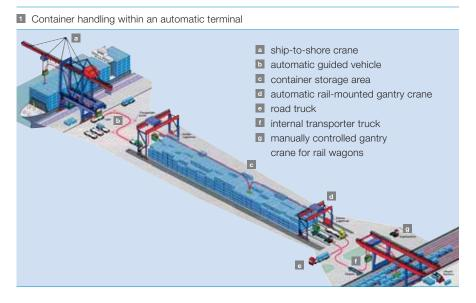
With modern ship-to-shore cranes a ship with 4000-5000 TEU (twenty feet equivalent) to unload/load can be handled in less than 24 hours
