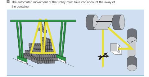
mum approach for the load, with rope lengths of 3–50 meters and with trolley and hoist speeds of 300 m/min and 200 m/min respectively.
