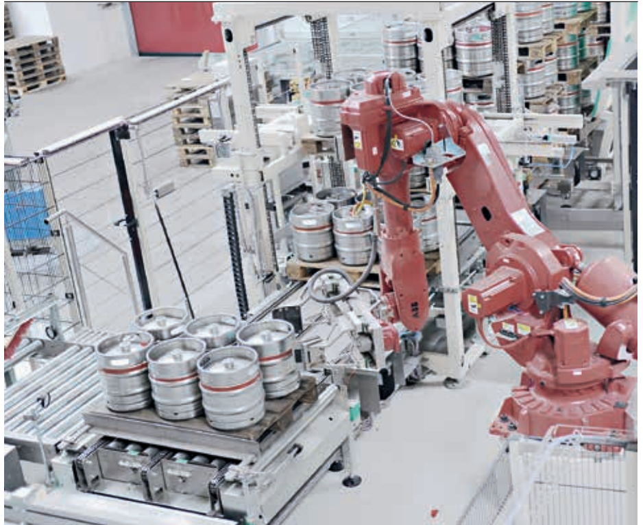
1 A robot stacking kegs concludes the chain of ABB automation that assists the beer maker.
