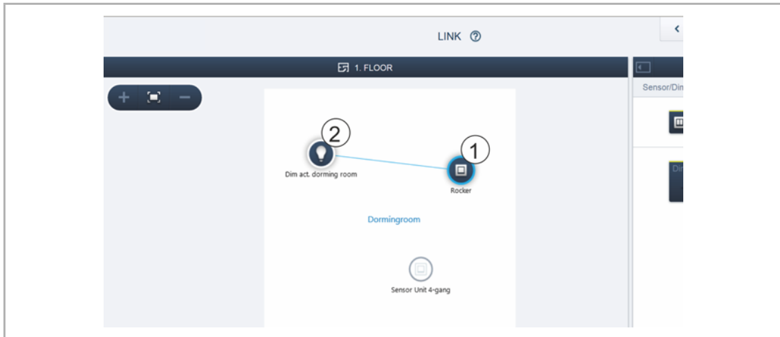
Fig. 21: Linking actuator and sensor
