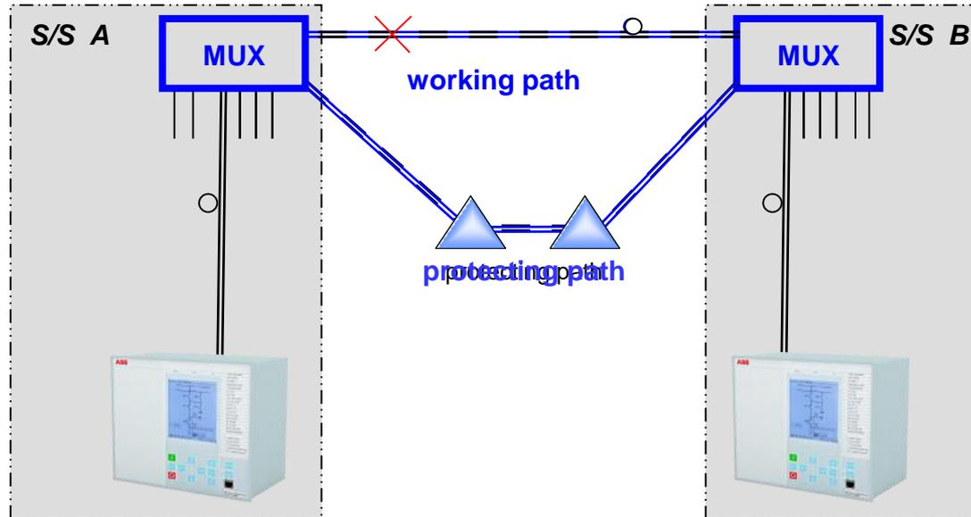
To avoid false tripping after switchover from working to protecting path protection services require:
