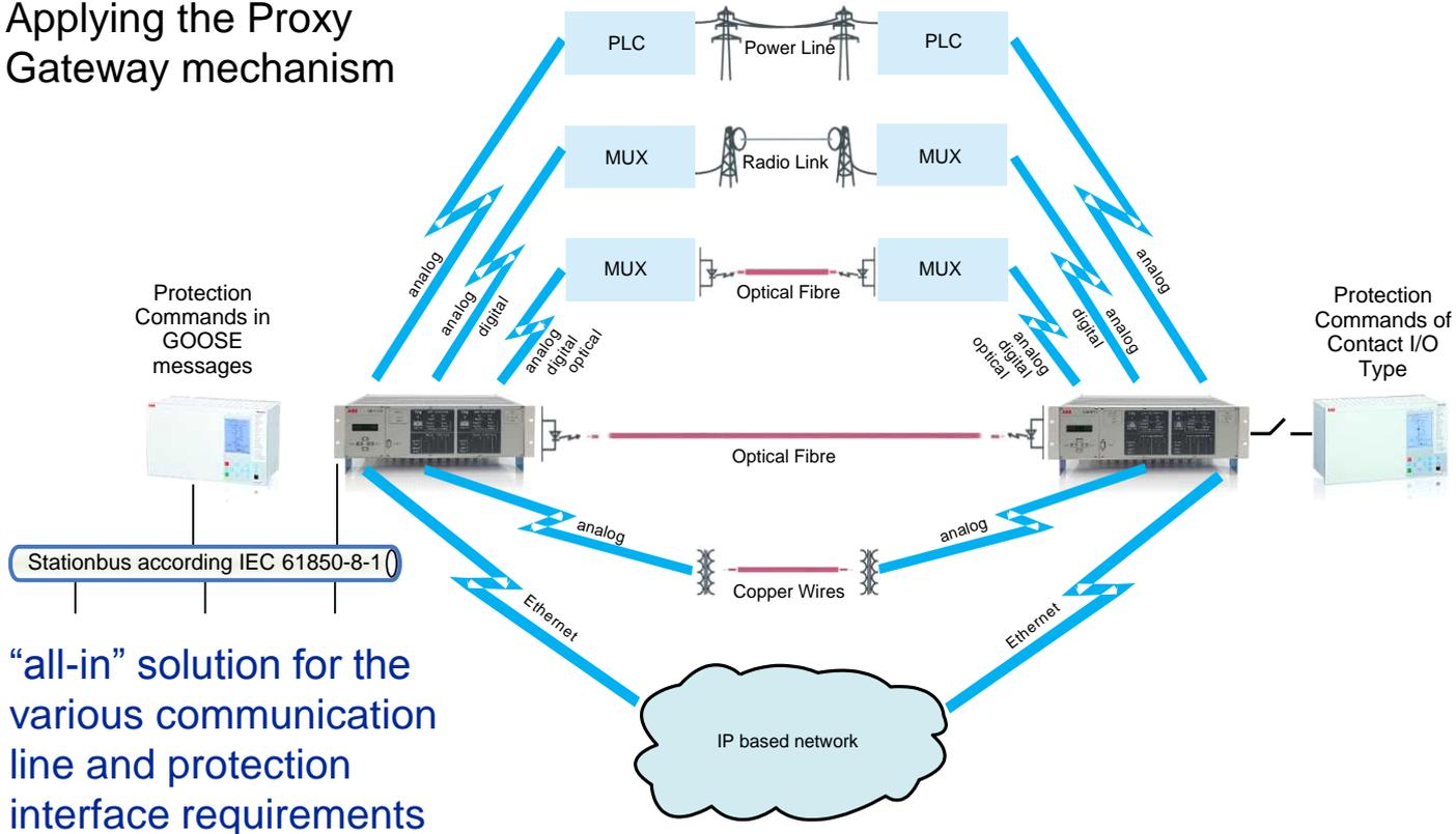
“all-in” solution for the various communication line and protection interface requirements
