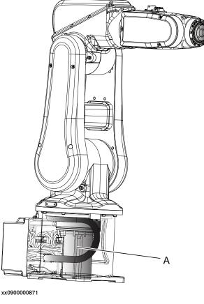
A Axis-1 motor with gearbox
