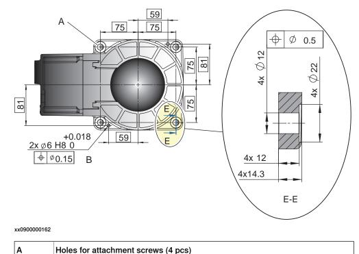
The illustration shows the hole configuration used when securing the robot.
