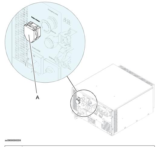
Brake release button (beneath the cover)
