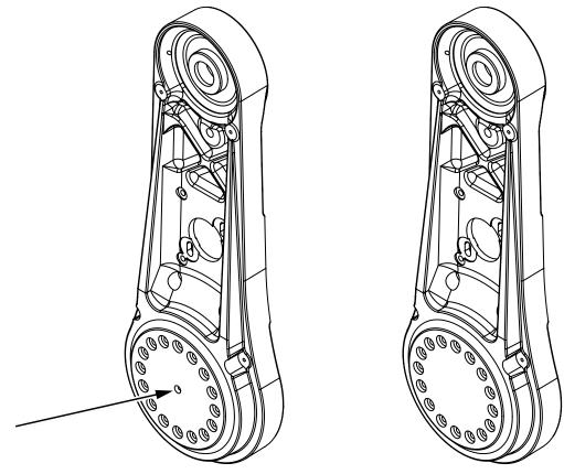
There are two different designs of the lower arm housing. One of the designs has an air release hole and the other does not.
