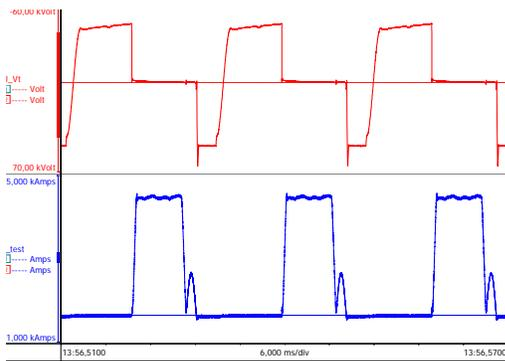
Figure 4 Periodic firing and extinction test / heat-run test (test set-up with two thyristor modules)
