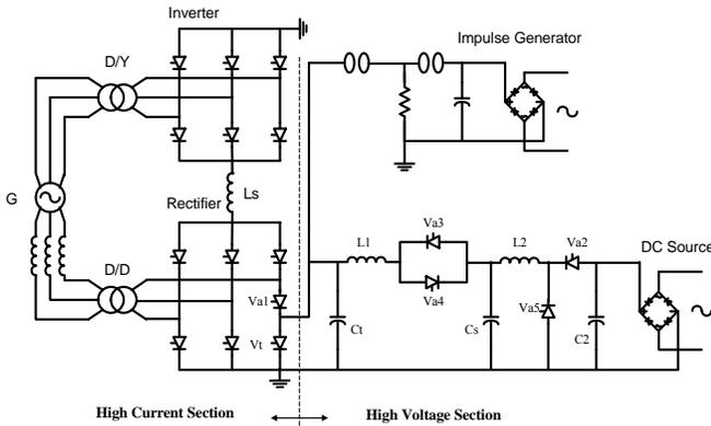
Figure 3 6-pulse back-to-back based synthetic test circuit
