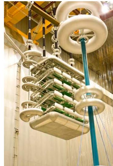
Figure 2 A high voltage MVU installed in the high voltage laboratory for dielectric test
