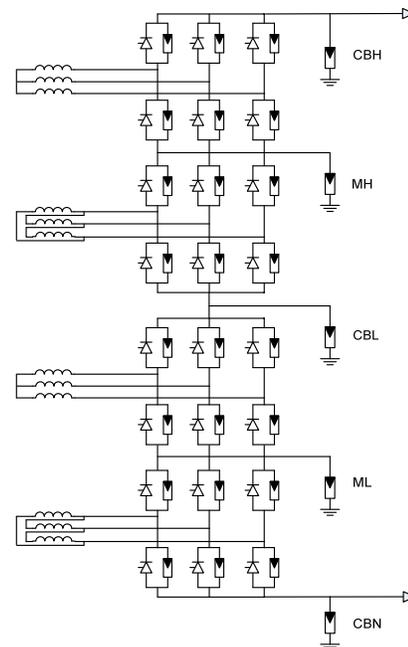
Figure 1 Converter valves and valve over-voltage protection scheme
