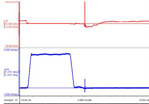
Figure 6 Tests with transient forward voltage during the recovery period
