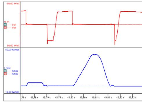
Figure 5 One-loop fault current with subsequent blocking voltage test
