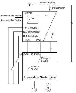
Figure 75 In this example the automatic pump alternation is in use.
