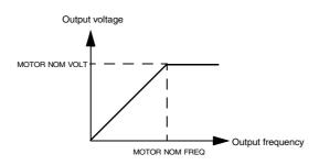
Figure 36 Output voltage as a function of output frequency.
