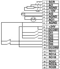
Reference voltage 10 VDC Actual signal; 0...20 mA (PID) Output frequency 0...20 mA <=> 0...52 Hz
