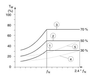
Figure 49 Underload curve types.  ${\rm T}_{\rm M}$  nominal torque of the motor,  $f_{\rm N}$  nominal frequency of the motor.
