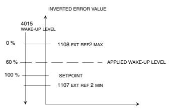
Figure 58 Example of how applied wake-up level floats with the set point, here parameter 4015 wake-up LeveL equals to 60 %, PID control inverted case.
