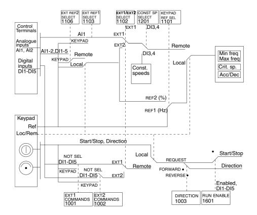
Figure 72 The control signal connections of the ABB Standard, Alternate and Premagnetise macros.
