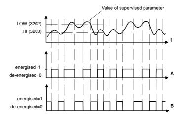
A = Parameter 1401 RELAY OUTPUT 1 (1402 RELAY OUTPUT 2) value is SUPRV1 OVER or SUPRV2 OVER.
