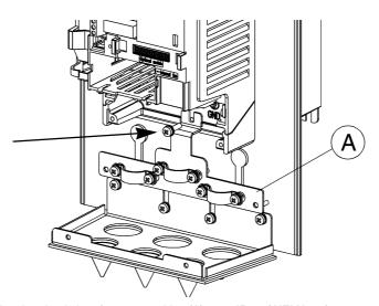
Figure 24 Fixing the gland plate for power cables (A), type IP 54 / NEMA12 frequency converters.
