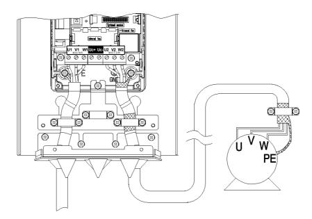
Figure 25 Motor cable connection for frame sizes R1 and R2 (IP 54 / NEMA12). Note! See "ACS 400 EMC Instructions" on page 157.
