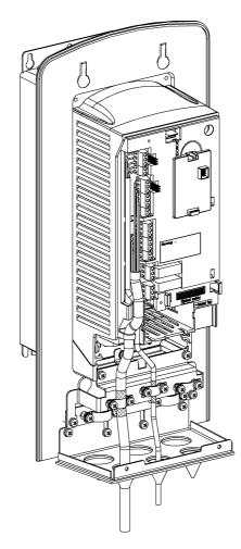
Figure 28 Control cable connections (IP 54 / NEMA12). Note! See "ACS 400 EMC Instructions" on page 157.
