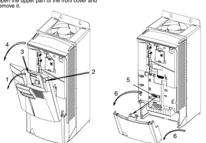
Figure 9 Opening the frame size R3 and R4 frequency converters of type IP 21 / NEMA1.
