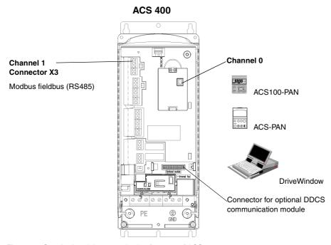
Figure 66 Standard serial communication features of ACS 400.
