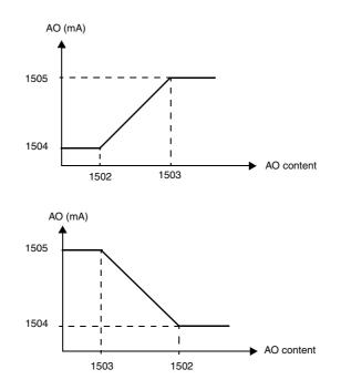
Figure 41 Analogue output scaling.
