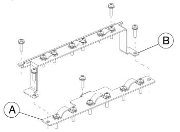
Figure 23 Gland plate for **power cables (A)** and for **control cables (B)**, type IP 54 / NEMA 12 frequency converters.
