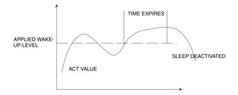
Figure 60 Wake-up level operation with inverted error value.
