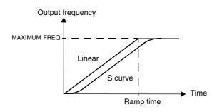
Figure 42 Definition of acceleration/deceleration ramp time.
