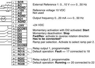
\*Note! DI 4 is used to configure ACS 400. It is read only once when power is connected. All parameters marked with \* are determined by the DI4 input.
