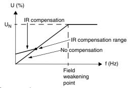
Figure 44 Operation of IR compensation
