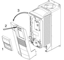
Figure 8 Opening the frame size R1 and R2 frequency converters of type IP 21 / NEMA1.
