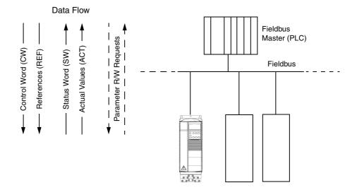
Figure 67 Structure of a fieldbus system.
