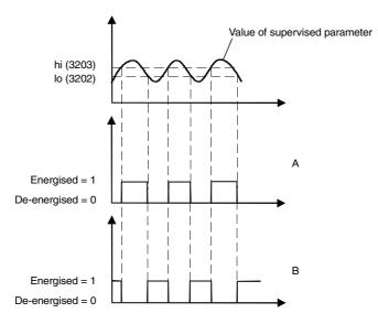
A = Parameter 1401 RELAY OUTPUT 1 (1402 RELAY OUTPUT 2) value is SUPRV1 OVER or SUPRV2 OVER
