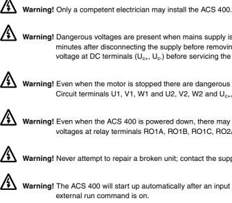
Warning! Dangerous voltages are present when mains supply is connected. Wait at least 5 minutes after disconnecting the supply before removing the cover. Measure the voltage at DC terminals  $(U_{c+}, U_{c-})$  before servicing the unit. See **E**.
