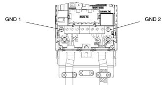
Figure 15 Removing the grounding screws from frame size R1 and R2 frequency converters.
