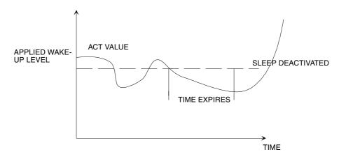
Figure 59 Wake-up level operation with non-inverted error value.
