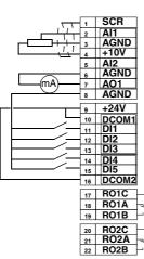
External Reference 1: 0...10 V <=> 0...50 Hz Reference voltage 10 VDC Not used Output frequency 0...20 mA <=> 0...50 Hz +24 VDC Start/Stop: Active to start ACS 400 Fwd/Rev: Activate to reverse rotation Constant Speed selection\* Constant Speed selection\* Premagnetise: Activate to start premagnetising Relay output 1, programmable Default operation: **Fault** => 17 connected to 18
