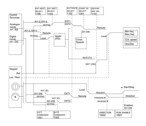
Figure 71 Selecting control location and control source.
