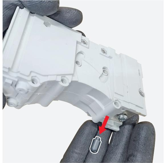
**39** By means of the pliers remove the silicone sheath located in the bottom part of the pole.
