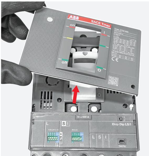
**7** By means of the cross screwdriver unscrew the 4 screws fixing the front cover to the circuit breaker main structure.
