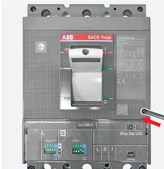
**5** Insert the flat screwdriver as shown in the picture and slightly push the screwdriver as shown by the arrow in order to raise up and to unhook the aesthetic front cover from circuit breaker main structure.
