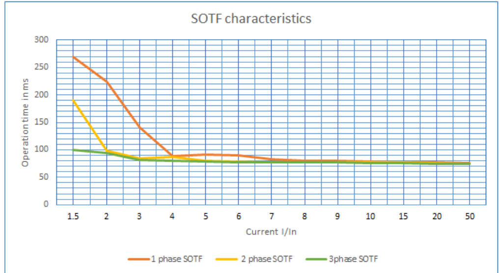
Figure 15: Switch-on to fault characteristics of relay REJ603
