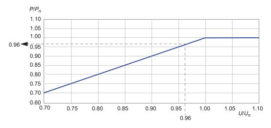
Example 1:  $P_n$  for ACS880-37-430A-7 is 400 kW. The input voltage (*U*) is 660 V. ->  $U/U_n$  = 660 V / 690 V = 0.96 ->  $P/P_n$  = 0.96 -> The derated power P = 0.96 × 400 kW = 384 kW.
