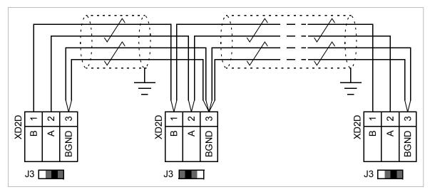
The diagram that follows shows the wiring of the drive-to-drive link. The diagram is applicable to these control units:
