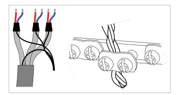
**Note:** At the other end of the cable, leave the shields unconnected or ground them indirectly via a high-frequency capacitor with a few nanofarads, eg. 3.3 nF / 630 V. The shield can also be grounded directly at both ends if they are in the same ground line with no significant voltage drop between the end points.
