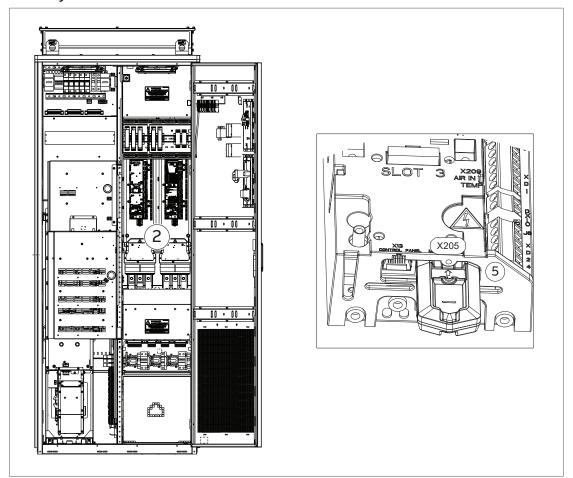
After you have installed a new memory unit or a software update, upload the parameter backup file to the control unit. Make sure that the software identifies the Drive rating ID. If the software does not identify the Drive rating ID, it cannot determine the voltage rating and the drive does not start.
