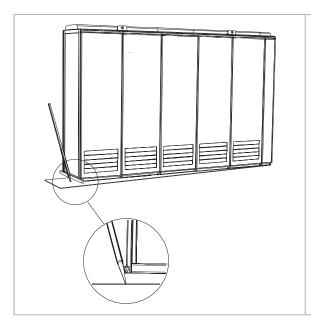
Move the cabinet into its final position with a slate bar (spud bar). Put a piece of wood between the edge of the cabinet and the bar to protect the cabinet frame.
