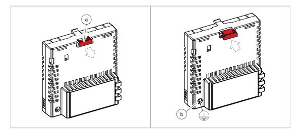
6. Connect the wiring to the module. Obey the instructions given in the documentation of the module.
