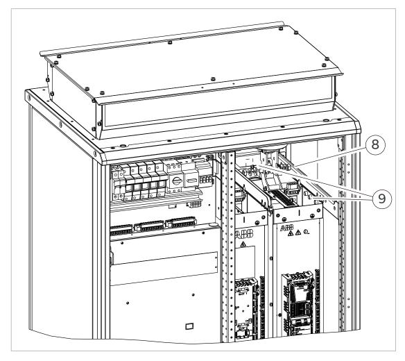
10. Pull the module out until the lifting eyes at each side of the module are accessible.
