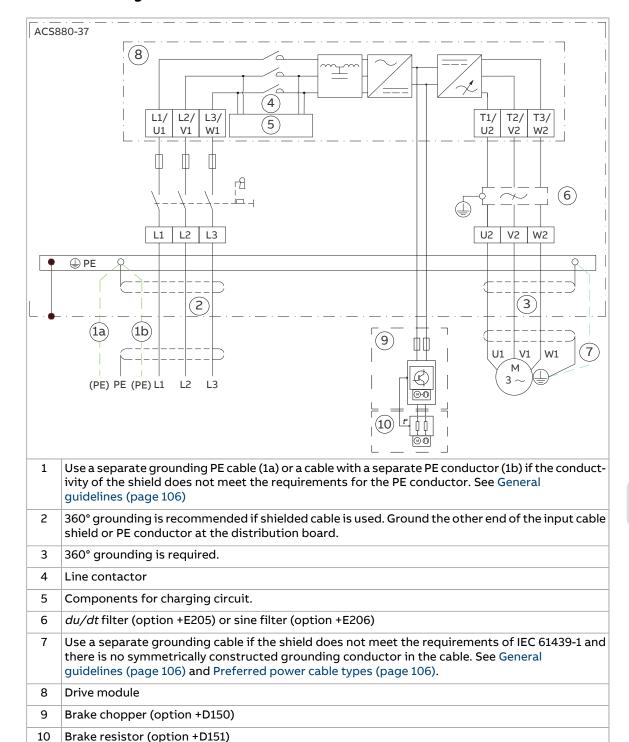
**Note:** If there is a symmetrically constructed grounding conductor on the motor cable in addition to the conductive shield, connect the grounding conductor to the grounding terminal at the drive and motor ends. Do not use an asymmetrically constructed motor cable. Connecting its fourth conductor at the motor end increases bearing currents and causes extra wear.
