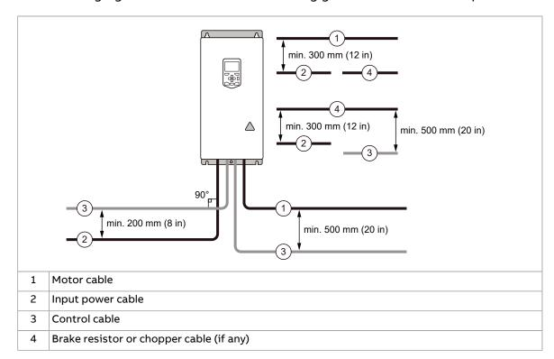
The following figure illustrates the cable routing guidelines with an example drive.
