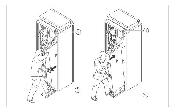
Make sure that the module does not fall over when you move it on the floor.
