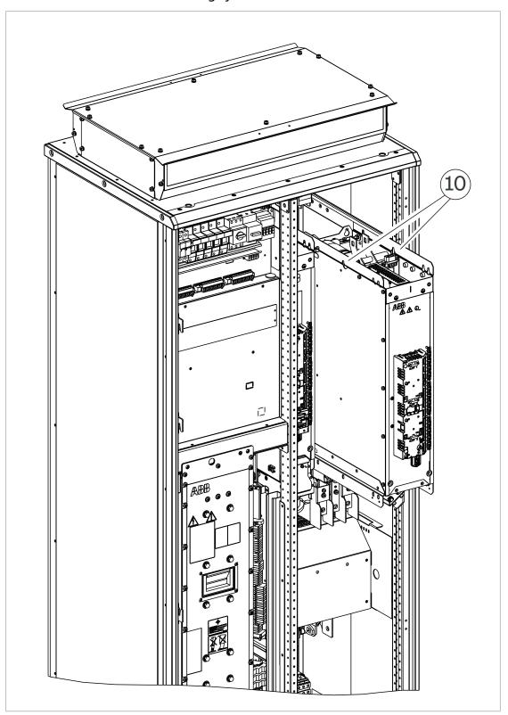
11. Attach a hoist to the lifting eyes and pull the module out. Install a new module in reverse order.
