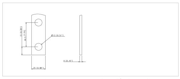
Distance between adjacent terminals is 25 mm (0.98 in) for drives without option +E202 and 50 mm (1.97 in) for drives with option +E202.
