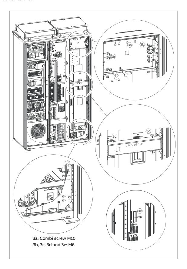
To open the module section swing-out frame, undo the M10 bolts from top and bottom (4 pcs).
