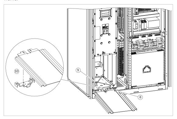
12. Pull the module carefully out of the cabinet along the ramp. While you pull the handle, keep a constant pressure with one foot on the base of the module to prevent the module from falling on its back.
