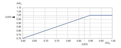
Example 1:  $P_n$  for ACS880-37-650A-3 is 355 kW. The input voltage (*U*) is 350 V. ->  $U/U_n$  = 350 V / 400 V = 0.875. ->  $P/P_n$  = 0.975 -> The derated power P = 0.975 × 355 kW = 346 kW.
