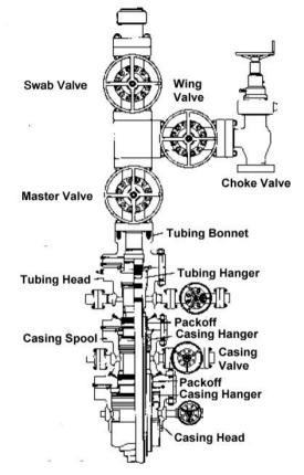
**Wing valve**. The wing valve can be a gate or ball valve. When shutting in the well, the wing gate or valve is normally used so that the tubing pressure can be easily read.
