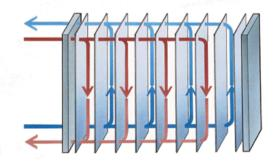
Heat exchangers of various forms are used to cool the gas. Plate heat exchangers (upper picture) consist of a number of plates where the gas and cooling medium pass between alternating plates in opposing directions. Tube and shell exchangers (next picture) place tubes inside a shell filled with cooling fluid. The cooling fluid is often pure water with corrosion inhibitors.
