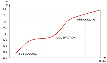
Figure 13. LNG Q/T diagram
