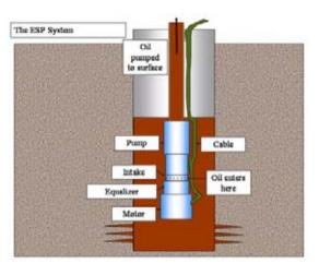
Installations down to 3.7 km with power up to 750 kW have been installed. At these depths and power ratings, medium voltage drives (up to 5kV) must be used.
