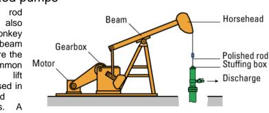
motor drives a reciprocating beam, connected to a polished rod passing into the tubing via a stuffing box. The sucker rod continues down to the oil level and is connected to a plunger with a valve.
