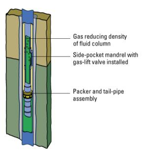
pressure ranges can be used to improve lifting and startup. III: Schlumberger oilfield glossary
