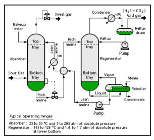
A typical amine gas treating process (as shown in the flow diagram) consists of an absorber unit, a regenerator unit and accessory equipment. In the absorber, a "lean" amine solution absorbs H2S and CO2 from the upflowing sour gas to produce a sweetened gas stream as a product. The "rich" amine solution contains the absorbed acid gases and is routed into the regenerator (a stripper with a reboiler). The stripped overhead gas from the regenerator is concentrated  $H_2S$  and  $CO_2$ .
