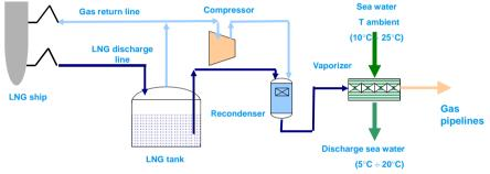
Figure 18. LNG terminal process overview
