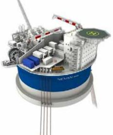
A variation of the FPSO is the Sevan Marine design. This uses a circular hull which shows the same profile to wind, waves and current, regardless of direction. It shares many of the characteristics of the ship-shaped FPSO, such as high storage capacity and deck load, but does not rotate and therefore does not need a rotating turret. *Photo: Sevan Marine*
