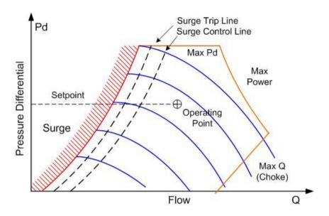
Figure 8. Compressor state diagram
