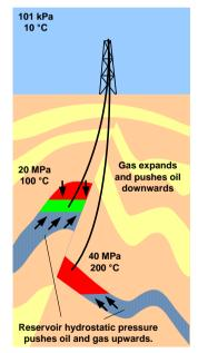
reservoir. The best reservoirs with advanced enhanced oil recovery (EOR) allow up to 70% recovery. Reservoirs can be quite complex, with many folds and several layers of hydrocarbon-bearing rock above each other (in some areas more than ten). Modern wells are drilled with large horizontal offsets to
