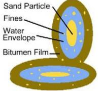
releases bitumen from the oil sand, and allows small air bubbles to attach to the bitumen droplets. The bitumen froth floats to the top of separation vessels, and is further treated to remove residual water and fine solids. It can then be transported and processed the same way as extra heavy crude.
