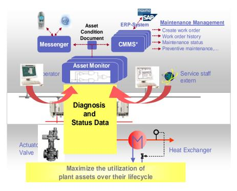
Figure 34. Computerized maintenance management system
