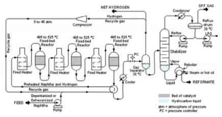
Figure 21. Catalytic reformer (Source: Wikipedia)
