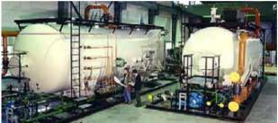
chlorides, come from the reservoir water and are also dissolved in the oil. The desalters will be placed after the first or second stage separator depending on GOR and water cut. *Photo: Burgess Manning Europe PLC*
