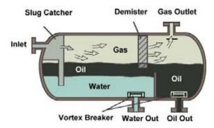
pressure reduction in a single separator will cause flash vaporization, leading to instability and safety hazards.
