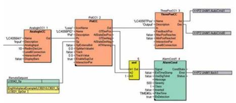
Figure 31. Function blocks define the control
