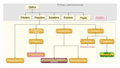
Figure 28. Olefins – propylene, derivatives
