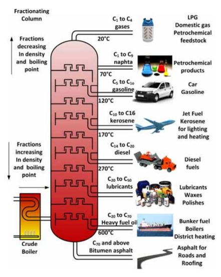
Figure 19. Fractionating continuous distillation, overview
