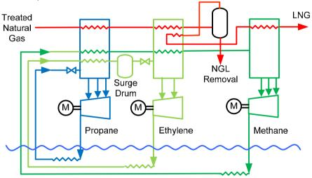
Figure 15. Optimized cascade process
