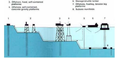
Figure 1. Oil and gas production facilities
