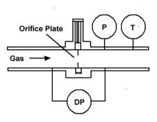
and ISO 5024/5167) to calculate normalized flow. Different ranges are accommodated with different size restrictions.
