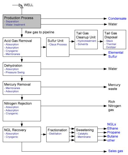
Figure 10. Typical gas plant
