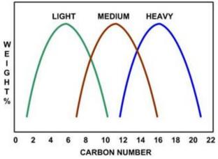
occurring 40 degrees API crude, fed to the distillation column at the refinery could come out of the still as 1.4 barrels of gasoline and naphtha (typically  $C_8H_{18}$ ), 0.6 barrels of kerosene (jet fuel  $C_{12-15}$ ), 0.7 barrels of diesel fuel (average  $C_{12}H_{26}$ ), 0.5 barrels of heavy distillate ( $C_{20-70}$ ), 0.3 barrels of lubricating stock, and 0.5 barrels of residue (bitumen, mainly poly-cyclic aromatics).
