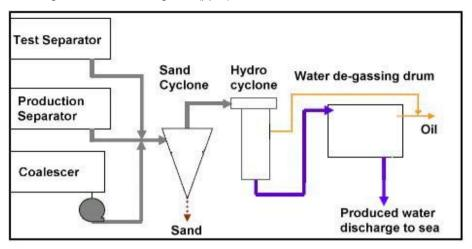
Figure 6. Produced water treatment
