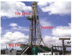
electric top drive hangs from the derrick crown and gives pressure and rotational torque to the drill string. The whole assembly is controlled by the drawworks. *Photo: Puna Geothermal Venture*
