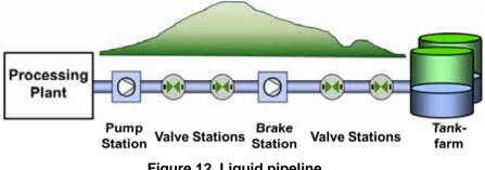
Figure 12. Liquid pipeline
