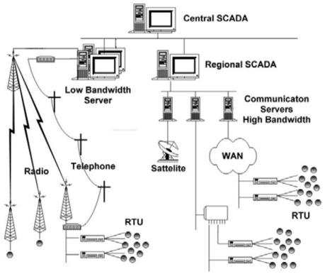
Figure 32. SCADA system topology (typical)
