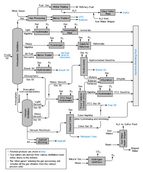
Figure 20. Refinery process flow diagram (Source: Wikipedia)
