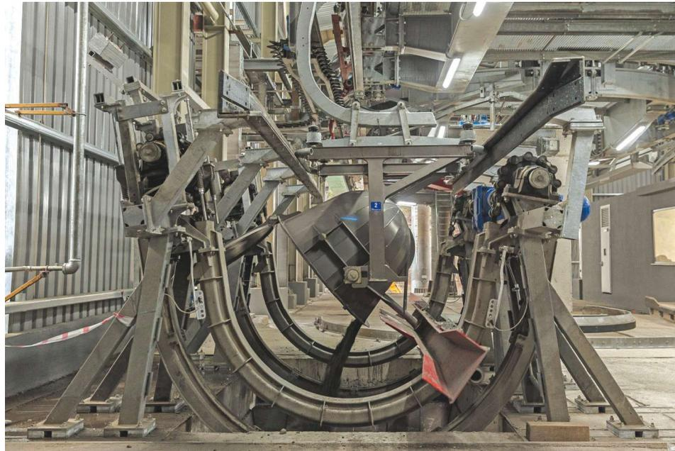
Buckets are opened, tipped and dumped automatically. (Photo: Doppelmayr)
