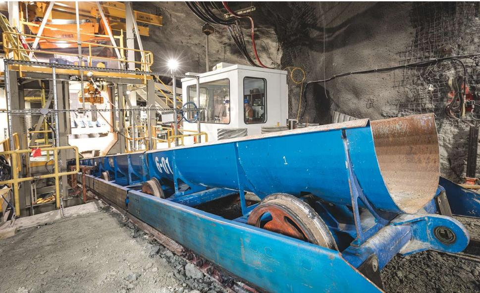
Low-profile steel cars in either 30 in. or 48 in. widths are linked together with a spill-proof connection to create a continuous U-shaped trough. (Photo: Agnico Eagle)
