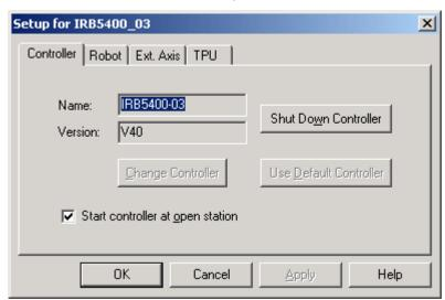
In the Setup for IRB5400\_03 dialog, click the Ext. Axis tab.
