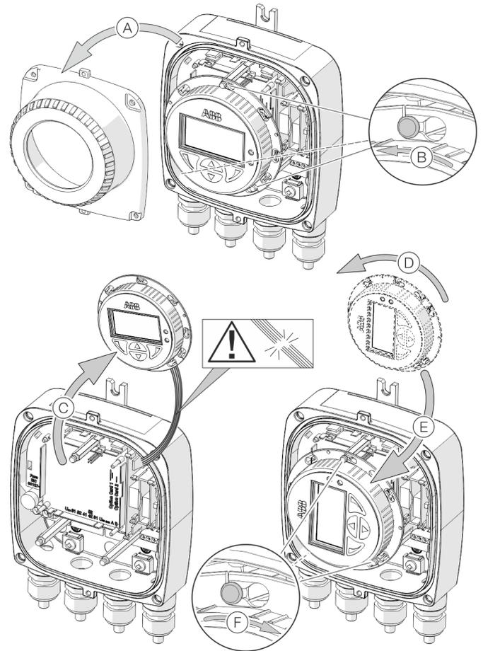
Figure 25: Rotating the LCD indicator
