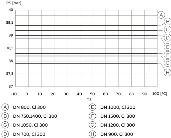
Figure 104: ASME flange, stainless steel, DN 700-1500, CI 300, B16.47 Series A, 1 x DN lay length
