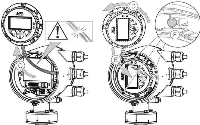
Figure 23: Rotating the LCD indicator
