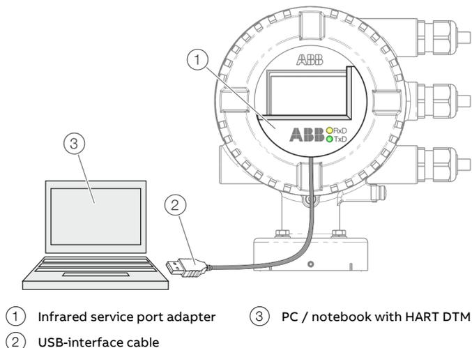
Figure 79: Infrared service port adapter on the transmitter (example)
