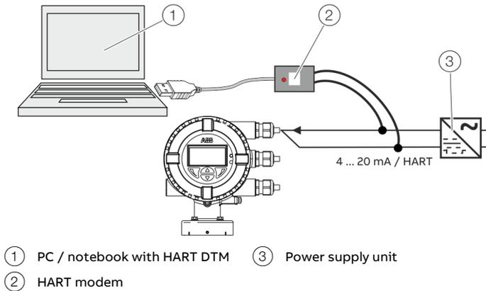
Figure 80: HART Modem on the transmitter (example)
