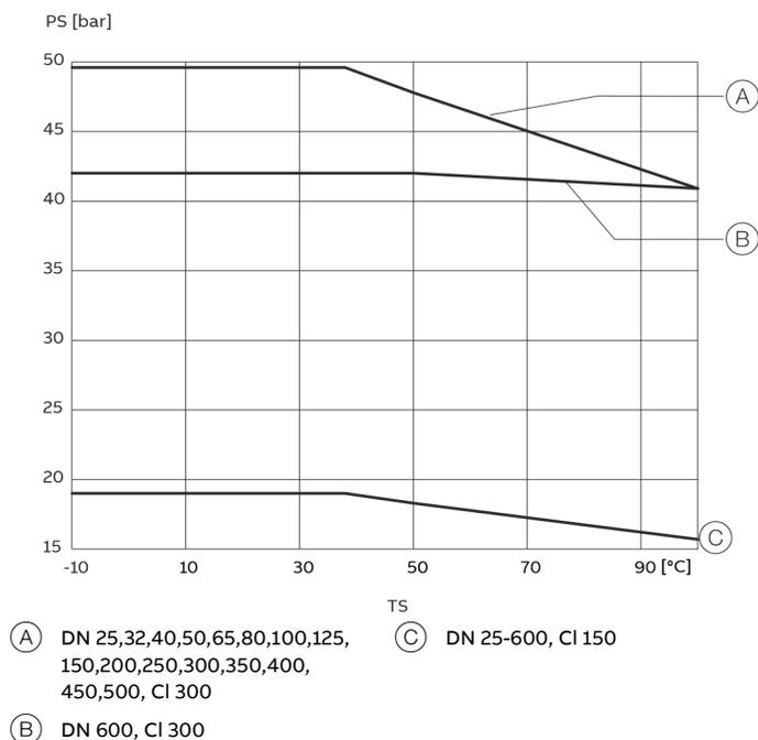
Figure 101: ASME flange B16.5, stainless steel, DN 25-600
