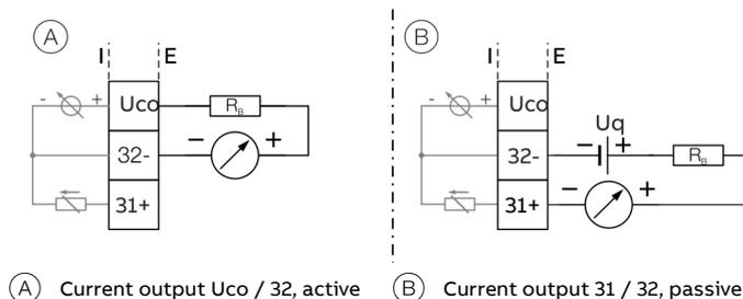
Figure 40: (I = internal, E = external,  $R_B$  = load)
