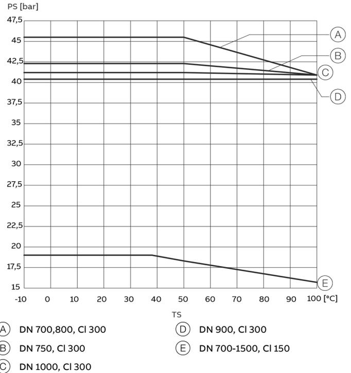
Figure 106: B16.47 Series B, ASME flange, stainless steel, DN 700-1500, 1.3 x DN lay length
