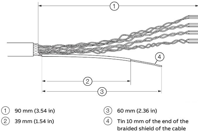
Figure 67: Preparing the EtherNet Cat5e cable
