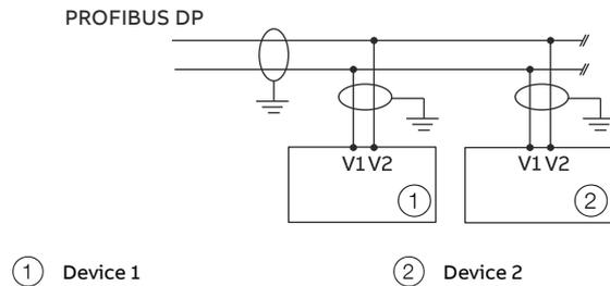
Figure 60: Communication with the PROFIBUS DP protocol
