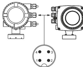
Figure 63: Pin assignment\* PROFIBUS PA M12-Plug (option)
