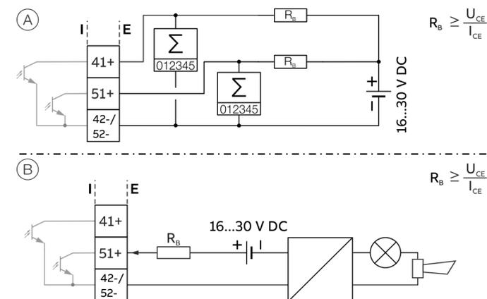
(A) Digital output 41 / 42, 51 / 52 passive as a pulse or frequency output
