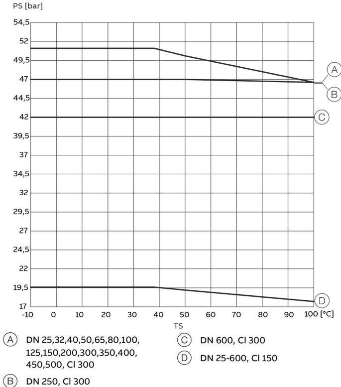
Figure 96: B16.5 ASME flange, carbon steel, DN25-600
