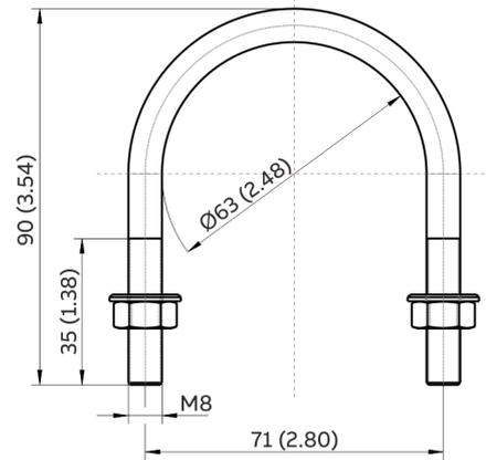
Figure 18: Assembly set for 2 in pipe mounting
