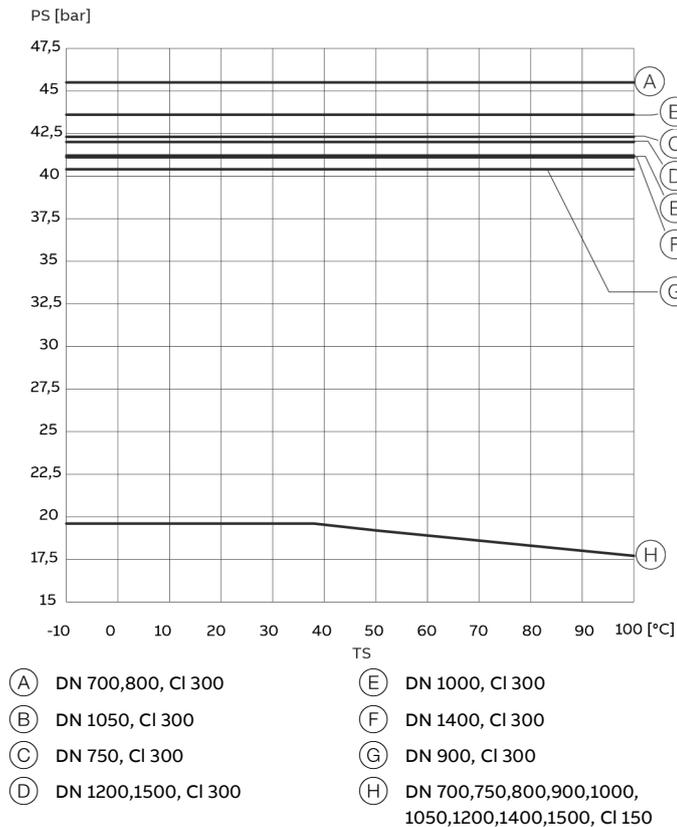
Figure 100: B16.47 Series B, ASME flange, carbon steel, DN 700-1500, 1.3 x DN lay length
