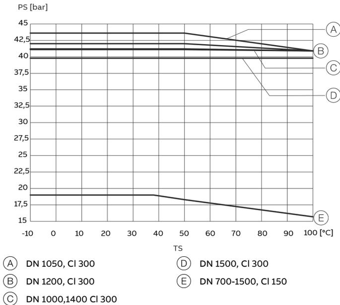
Figure 105: B16.47 Series A, ASME flange, stainless steel, DN 700-1500, 1.3 x DN lay length
