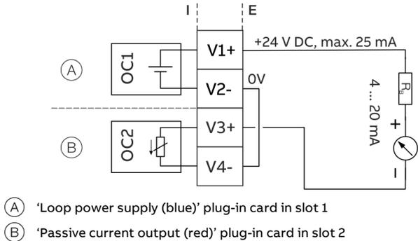
Figure 52: Active current output V3 / V4 (example)
