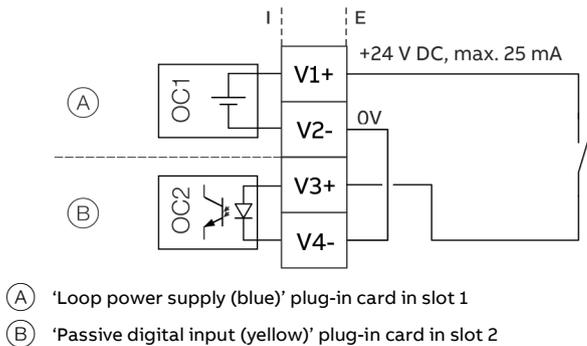
Figure 53: Active digital output V3 / V4 (example)
