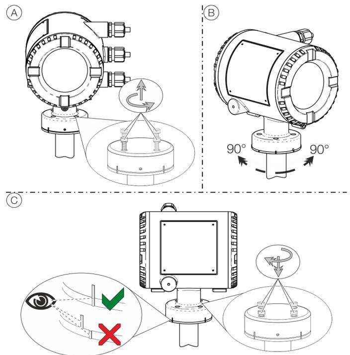
Figure 22: Rotate transmitter housing
