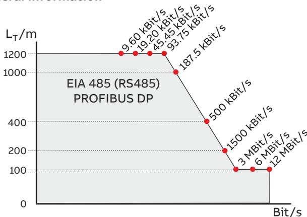
Figure 61: Bus cable length depends on the transmission rate
