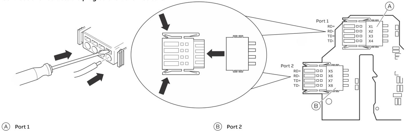
**Figure 66: Ethernet card connection**
