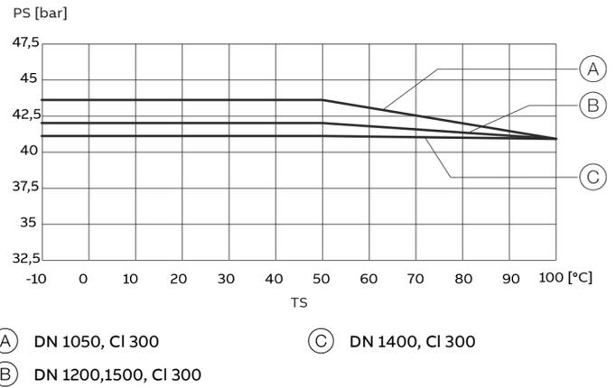
Figure 107: B16.47 Series B, ASME flange, stainless steel, DN 700-1500, 1.3 x DN lay length
