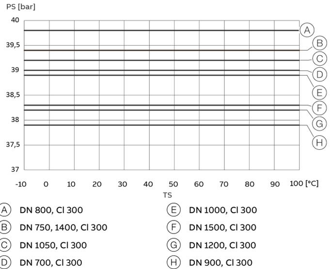
Figure 98: ASME flange, carbon steel, DN 700-1500, CI 300, B16.47 Series A, 1 x DN Lay Length
