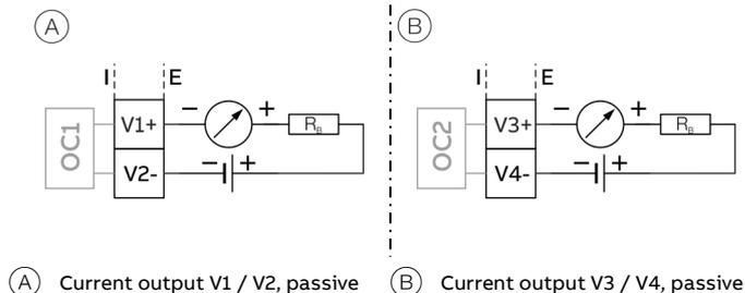
Figure 43: (I = internal, E = external, R<sub>B</sub> = load)
