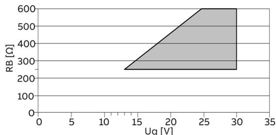
Permissible source voltage U<sub>q</sub> for passive outputs in relation to load resistance R<sub>B</sub> where I<sub>max</sub> = 22 mA. ■ = Permissible range
