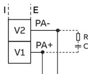
Figure 62: Communication with the PROFIBUS PA protocol
