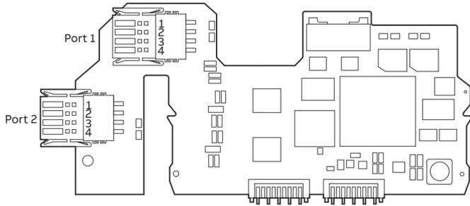
Figure 64: Ethernet communication plug-in card
