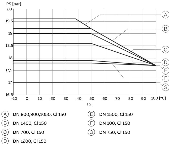
Figure 97: ASME flange, carbon steel, DN 700-1500, CI 150, B16.47 Series A, 1 x DN Lay Length
