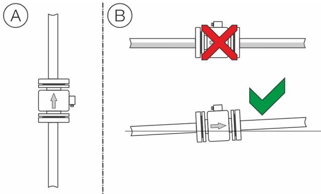
Figure 8: Mounting position
