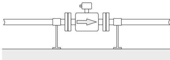
Figure 6: Flow direction
