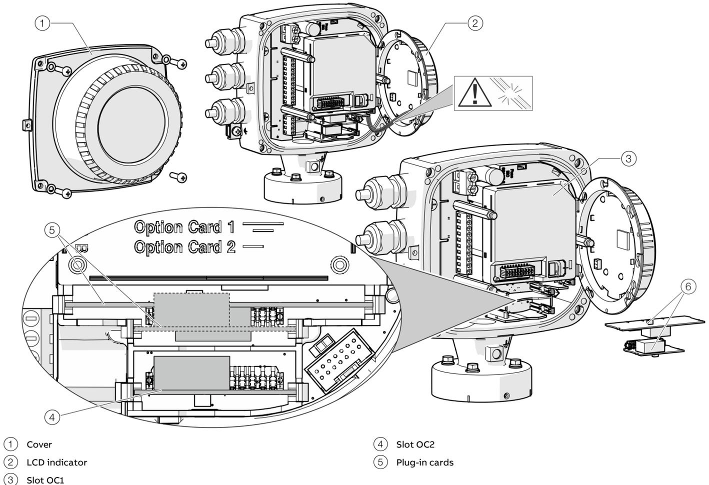
Figure 27: Installation of plug-in cards (example, single-compartment housing)
