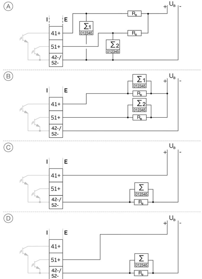
Figure 54: Connection versions digital output 41 / 42 and 51 / 52
