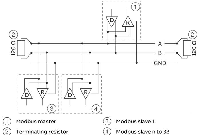
Figure 59: Communication with the Modbus protocol
