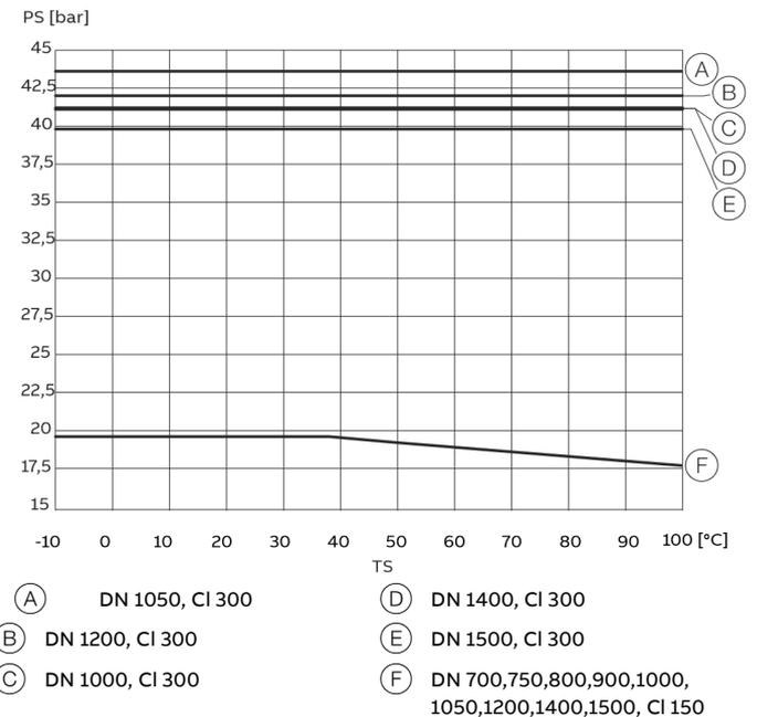
Figure 99: B16.47 Series A, ASME flange, carbon steel, DN 700-1500, 1.3 x DN lay length
