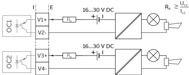
Figure 45: Plug-in card as binary output (I = internal, E = external,  $R_B$  = load)
