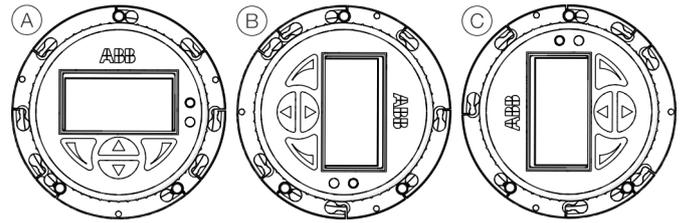
Figure 24: Possible positions of LCD indicator
