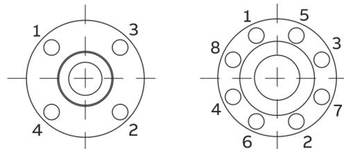
Figure 16: Tightening sequence for the flange screws
