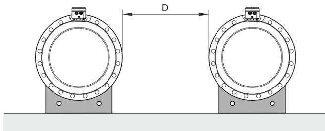
Spacing  $D \geq 1.0 \text{ m}$  (3.3 ft) for Design Level 'A'
