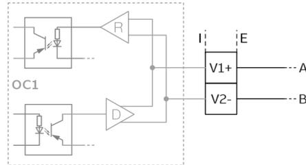
Figure 48: Plug-in card as a Modbus / PROFIBUS DP/PA interface (I = internal, E = external)
