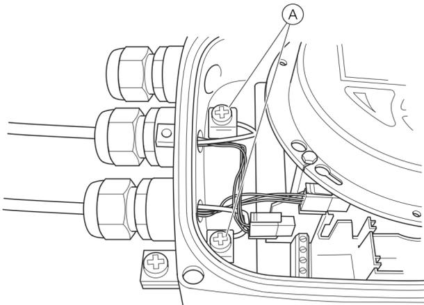
Figure 68: Ground the Ethernet connection cable
