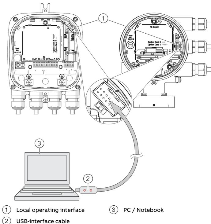
Figure 78: Connection to the local operating interface
