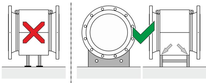
Figure 5: Support for nominal diameters greater than DN 400
