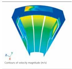
location of hot spots in the event of motor overload, which helped identify areas in which modifications were made to improve cooling and reduce losses.
