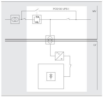
The PCS100 MV UPS can be installed to protect the complete supply or just selected sensitive loads → 1. In a data center this could include the mechanical loads → 2. Installing the UPS protection at the MV level provides the most energy efficient configuration as the lower currents at this voltage result in lower losses.
