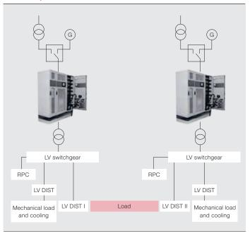
3 Single-conversion topology is a natural choice for MV. Power electronics and power storage can remain at LV with transformer coupling to MV.
