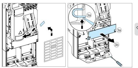
Note: Drive with cable box is used as an example in the figure. Cable box is optional and need to be ordered separately.
