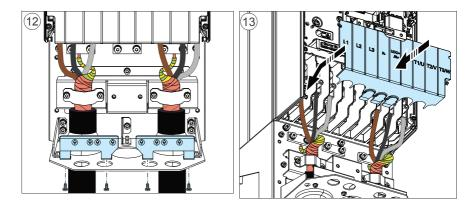
Note: Drive with cable box is used as an example in the figure. Cable box is optional and need to be ordered separately.
