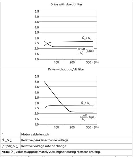
**Note:** Due to installation, cable types and motor impedance, the worst case value may be higher than the estimate value (curve).
