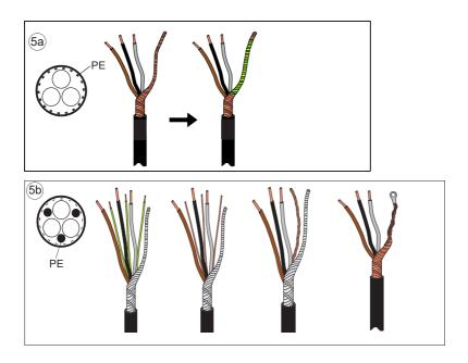
7. Connect the input power cable. Use terminals L1, L2 and L3. Tighten the screws to the torque given in the table.
