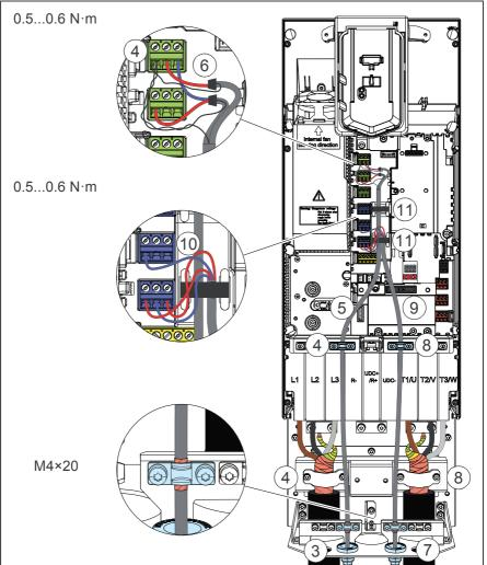
Note: Drive with cable box is used as an example in the figures. Cable box is optional and need to be ordered separately.
