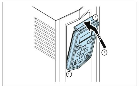
To reinstall the control panel, put the bottom of the container in position (1), press the retaining clip at the top (2) and push the control panel in at the top edge (3).
