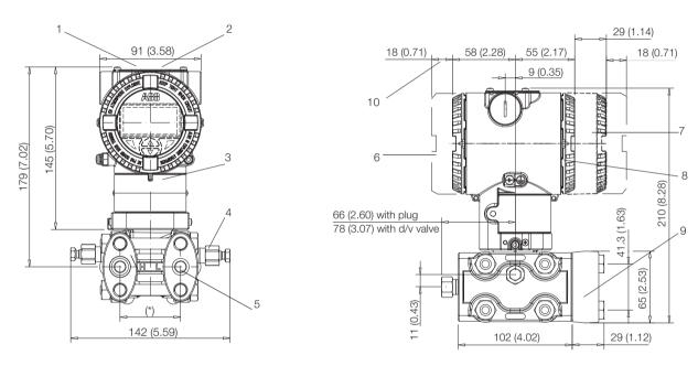
(\*) FOR MODEL 266DSH: 54 (2.13) mm (in) on 1/4 – 18 NPT process flange
