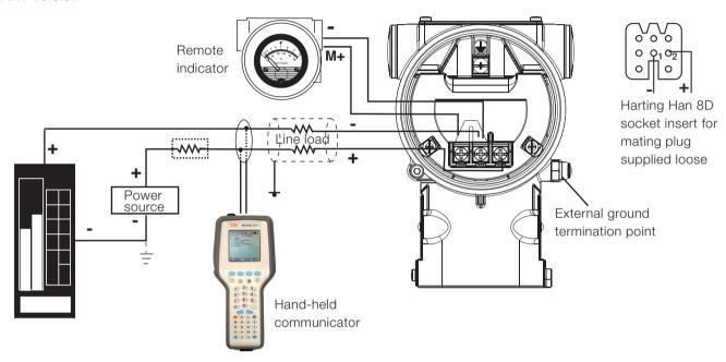
HART hand-held communicator may be connected at any wiring termination point in the loop, providing the minimum resistance is 250 ohm. If this is less than 250 ohm, additional resistance should be added to allow communications.
