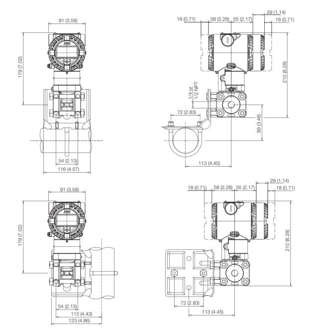
Transmitter with DIN aluminium housing - horizontal flanges on bracket for vertical or horizontal 60 mm (2in) pipe mounting
