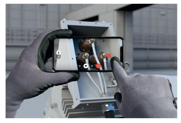
It is not always practical to have an ABB specialist physically at the site to fix a problem. On-site maintenance engineers can now call upon the help of ABB technical specialists using Visual Remote Support to help rapidly and efficiently navigate to the root of the problem.
