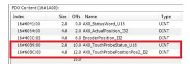
If you need to use digital input 1 or the negative edge (or both edges) of one of the fast inputs then simply add the necessary PDO mappings to access this data (again, refer to AN00221 for further information if required).
