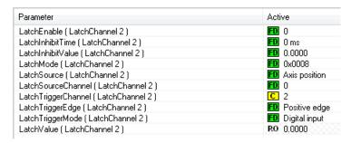
You can see that, by default, this channel is configured to capture Axis position (of Axis 0, as set by LatchSourceChannel) from a positive/rising edge of digital input 2 (where 2 is set by the LatchTriggerChannel).
