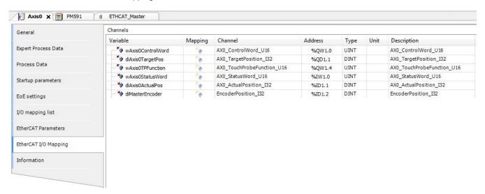
Save the project and launch CoDeSys (accept the confirmation to update the configuration). We can now create our master axis and use this mapped encoder to set the position of our master axis.
