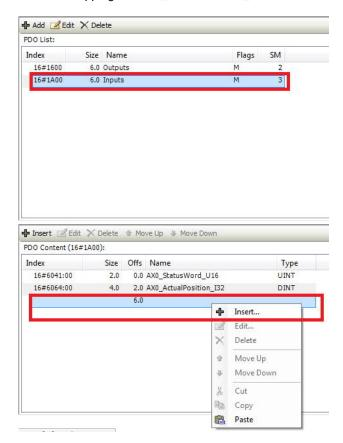
Now click on 'Insert...' and select Object 14#400C sub index 16#03 from the list of available objects (Object 16#400C is 'Encoder position' and the subindexes relate to each encoder channel.....subindex 16#01 is channel 0, subindex 16#02 is channel 1 and subindex 16#03 is channel 2).
