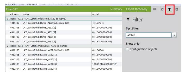
As we mentioned earlier, if you're using the drive for a master encoder you are unlikely to change the settings for LATCHSOURCE and LATCHSOURCECHANNEL, and the hardware connections will probably determine the LATCHTRIGGERCHANNEL, so it's most likely that you will use the Parameter Viewer to configure the "fixed settings" and SDO access for settings that the operator might want to adjust to suit a particular machine configuration.
