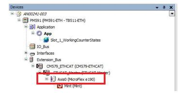
Double-click this icon to display the settings in the right-hand pane. "Enable Expert Settings" needs to be selected on the General tab (this should already be the case if you have used the project from AN00205 as the starting point or if you have opened the example included with this application note).
