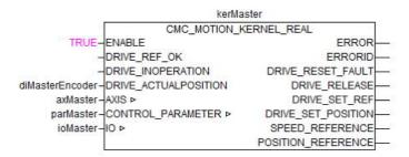
All of the code needed to create the master axis is now completed and the axMaster AXIS\_REF can now be used as the master axis for all of the available multi-axis PLCopen motion functions available within the PS552-MC-E motion libraries (e.g. MC\_GearIn, MC\_GearInPos, MC\_CamIn etc...).
