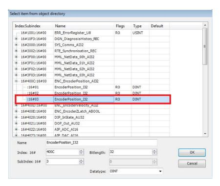
Click OK and this object will be added to the list of PDO mappings from the drive to the PLC.
