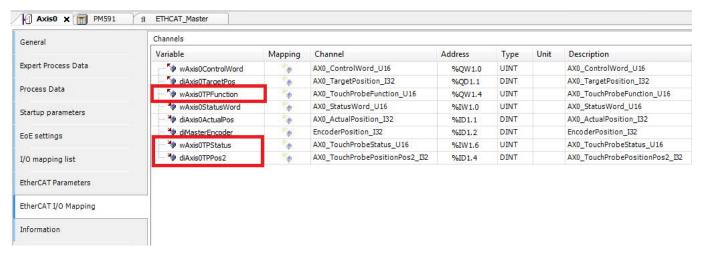
Make sure you are logged out of the PLC, add the required PDO mappings to the Automation Builder configuration as shown above and then right click the PLC application icon and select 'Create configuration data' to force the CoDeSys global variables to be updated to include definitions for our new PDO mappings.
