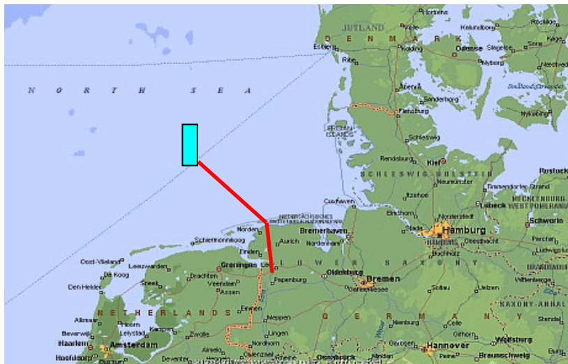
Figure 8. The BorWin 1 project in the North Sea connecting a 400 MW wind farm.
