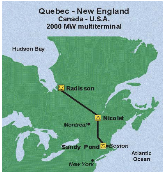
Figure 3.0 The HQ- NE Mutli-Terminal DC System
