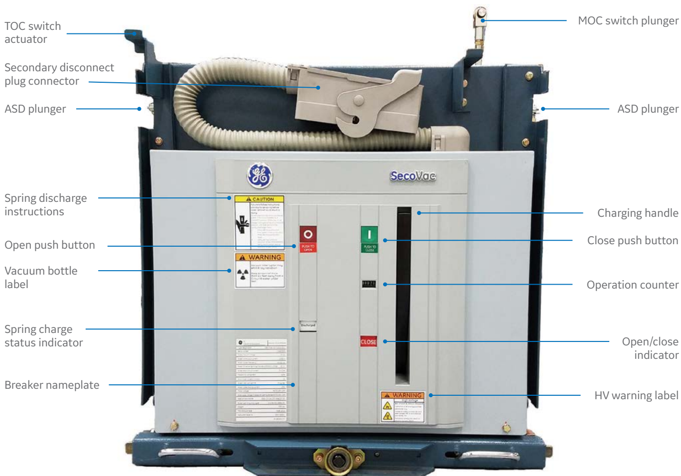
Figure 6: SecoVac VB2+ Vacuum Circuit Breaker
