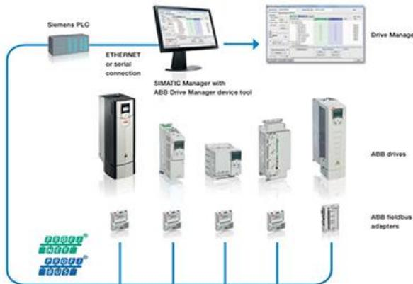
Drive Manager for SIMATIC (DM4S-01) is a plug-in device tool that can be easily installed into the STEP 7 and TIA Portal. It utilizes the TCI interface of the SIMATIC PLC to communicate with the drives connected to PROFIBUS or PROFINET network.
