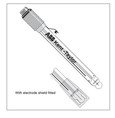
Fitted with low resistance 'blue glass' membrane, grooved cap for good grip, and integral replaceable refill stopper. Supplied with electrode shield 1160-206 for use if extra protection is required. Ideal for use in non-aqueous titrations.
