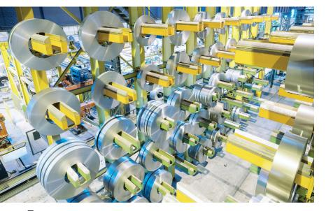
In order to further improve and secure the strip tension measurement in the CVC cold rolling mill, thyssenkrupp has upgraded to ABB Pressductor PillowBlock load cells with a 20-ton load capacity. This has eliminated the excessive building height, previously caused by undersized mechanical parts.
