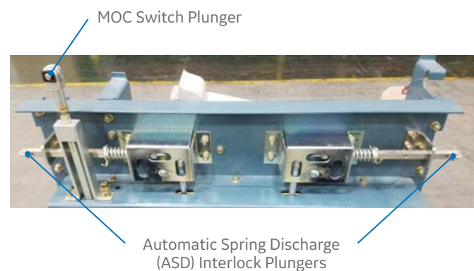
Figure 9: Automatic Spring Discharge (ASD) Interlock Plungers
