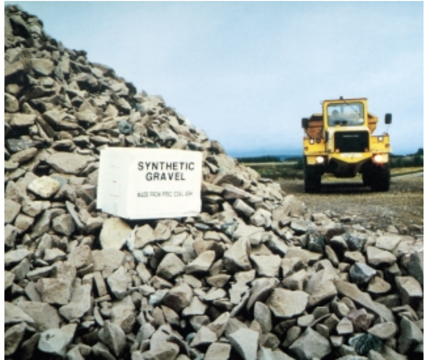
Synthetic gravel produced from PFBC ash
