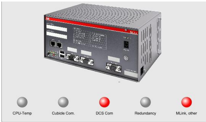
Fig. 75: MLink critical state signals
